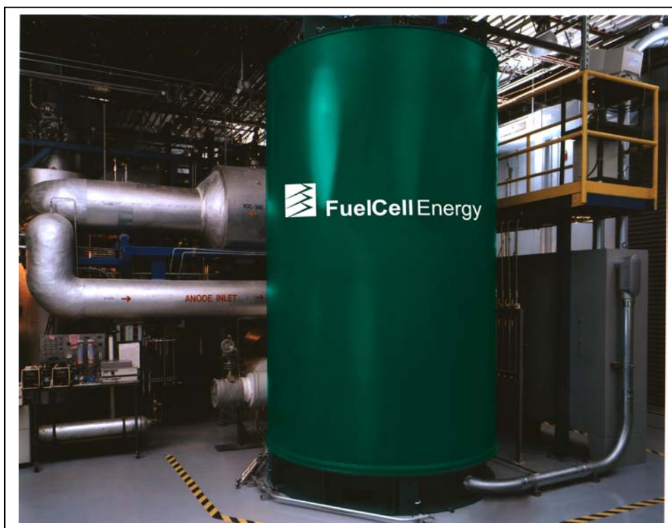
Figure 4. PRODUCT BUILDING BLOCK STACK DEMONSTRATION: MW-Class Product Stack Design is Founded on This Test
