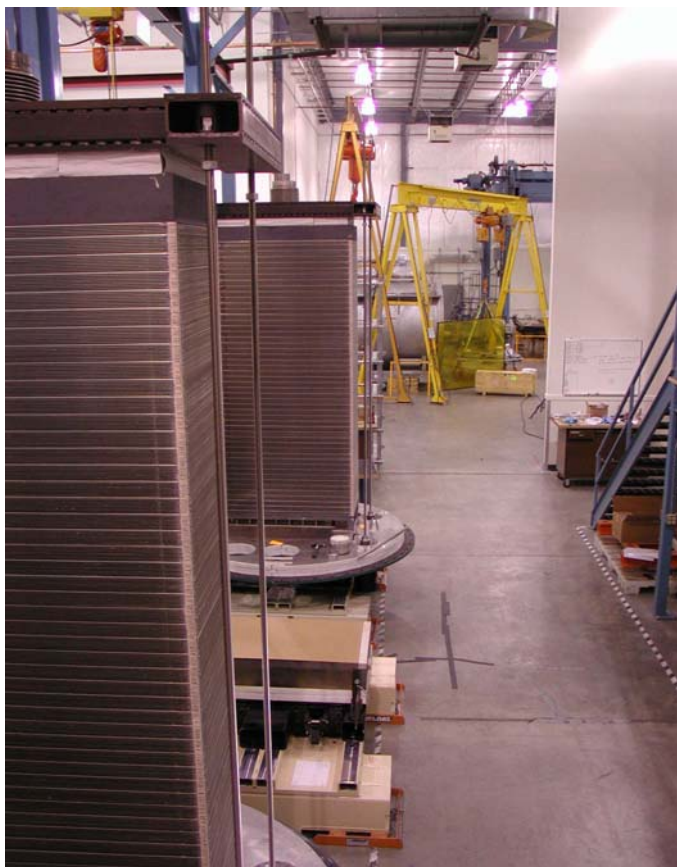
Figure 7. STACK FINAL ASSEMBLY FACILITY: Capable of Assembling Two Stacks Simultaneously
