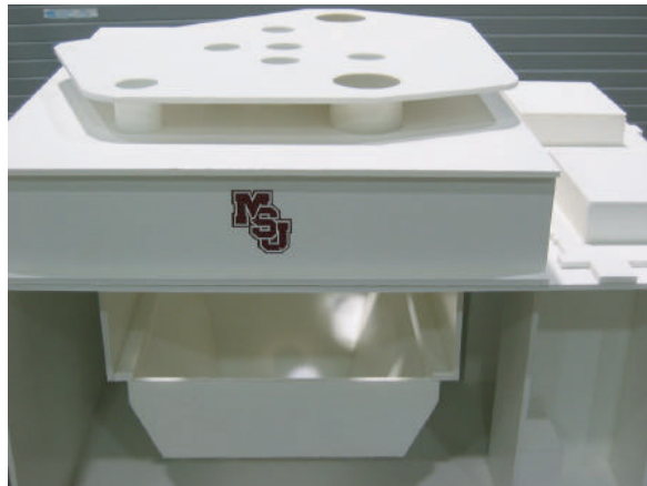
FIGURE 7. One-fifth-scale foam model of WVNS melter.
