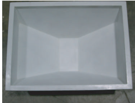
FIGURE 8. One-fourth-scale mock-up of WVNS melter core assembly.
