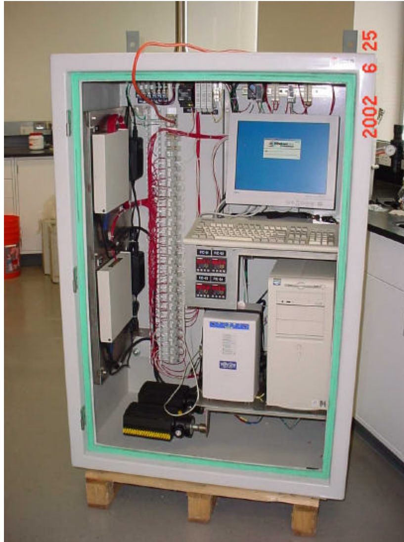
Figure 4-6. Photograph of Pilot Unit Control Panel Prior to Installation on Pilot Skid
