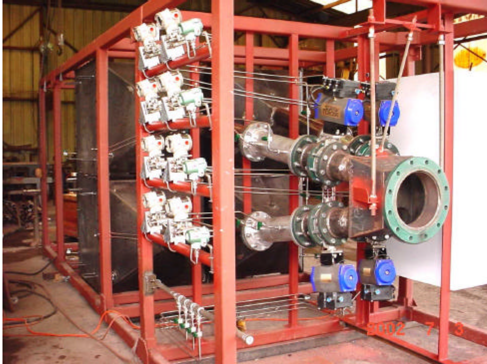
Figure 4-5. Photograph of the Pilot Skid from the Exit End, Near the Completion of its Mechanical Fabrication
