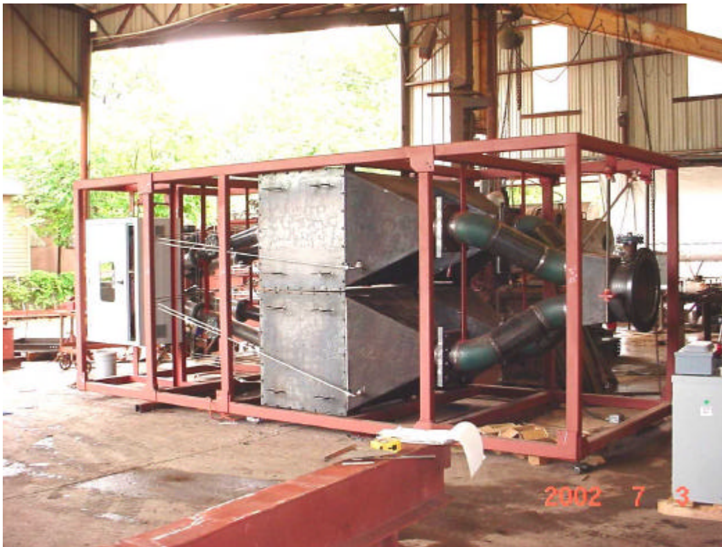
Figure 4-4. Photograph of the Pilot Skid from the Side on the Inlet End, Near the Completion of its Mechanical Fabrication
