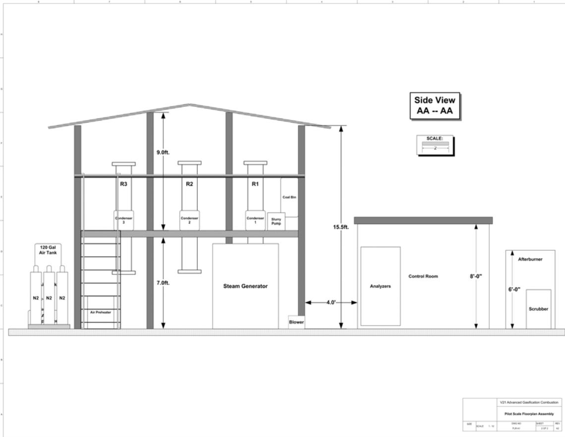
Figure 14. Pilot-scale floor plan (side view).
