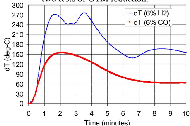
Figure 11. Comparison of temperature increase during OTM oxidation step for two tests with different OTM reduction feeds.
