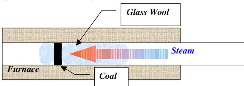
Figure 2. Experimental system configuration: relative positions of coal and glass wool packing material.
