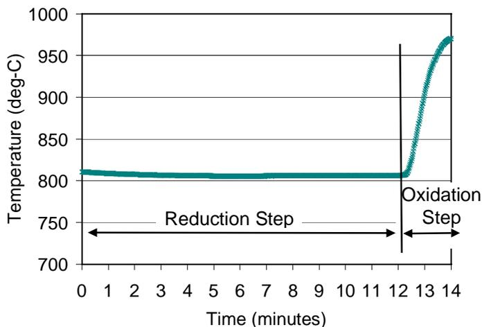
Figure 5. Temperature profile during reduction and oxidation steps of OTM test.
