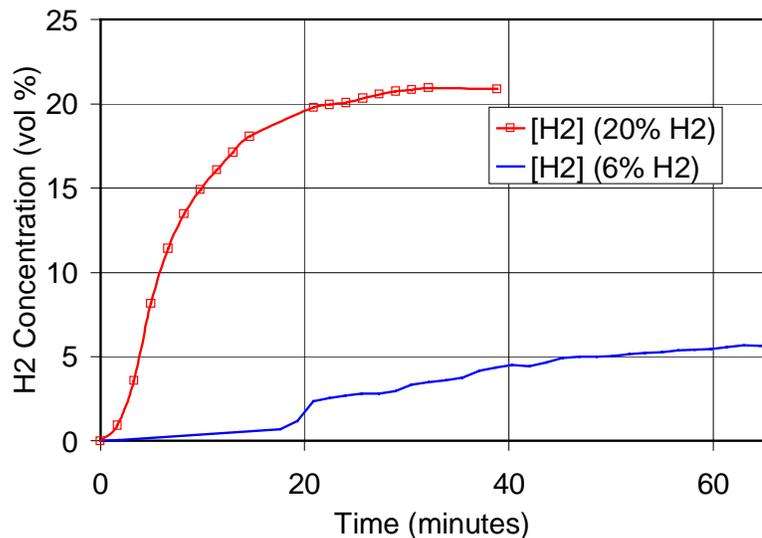
Figure 8. H<sub>2</sub> concentration during OTM reduction step for two different H<sub>2</sub> feed concentrations.
