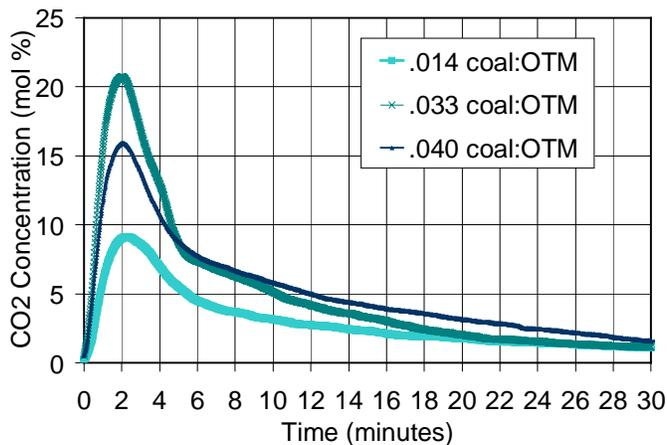
Figure 6. CO<sub>2</sub> concentrations during the reduction step of OTM tests for three different coal:OTM ratios.
