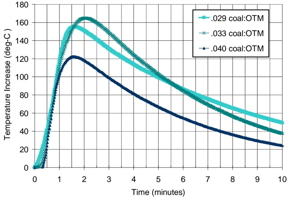
Figure 7. Temperature increase during oxidation step of OTM tests for three different coal:OTM ratios.
