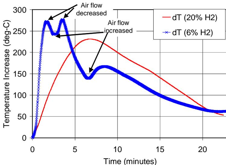
Figure 9. Temperature increase during OTM oxidation step for two different H<sub>2</sub> concentration tests.
