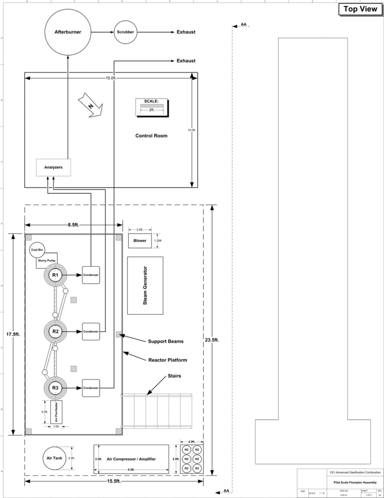
Figure 13. Pilot-scale floor plan (top view).
