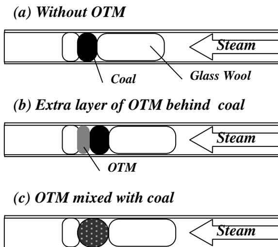
Figure 3. Arrangement of OTM relative to coal (layered or mixed).
