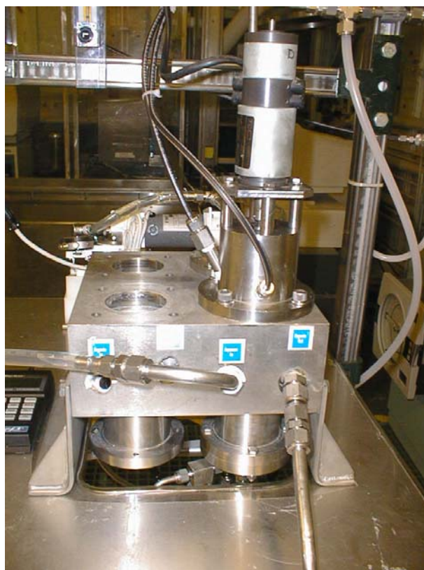
Figure 3. 5.5-cm centrifugal contactor “four-pack” configured for testing of a single stage.
