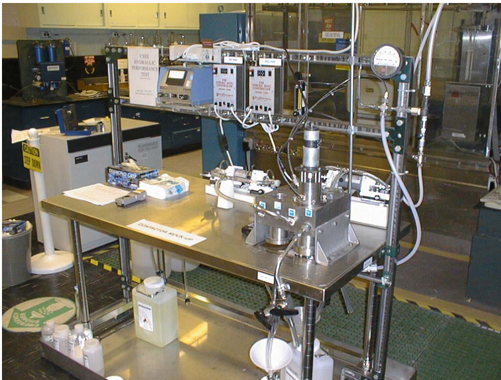
Figure 2. 5.5-cm diameter centrifugal contactor test setup.
