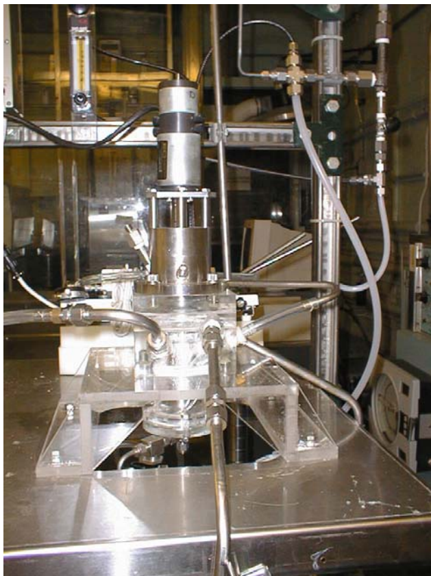
Figure 15. Single stage 5.5-cm centrifugal contactor with Plexiglas® housing.
