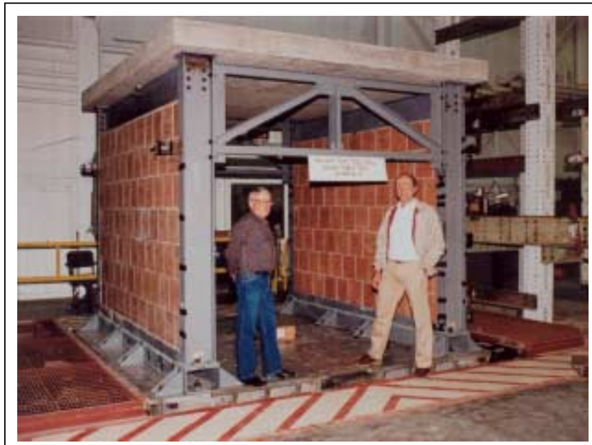
FIG. 6. Shake-table Test Setup
