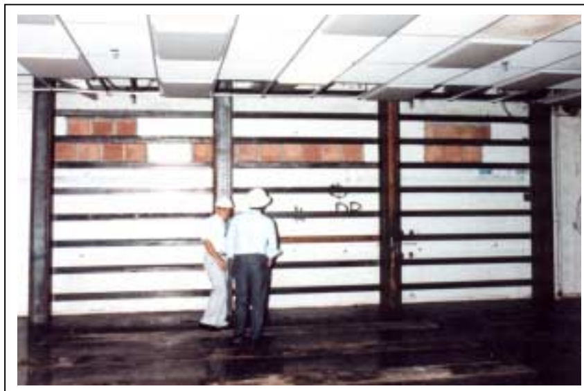
FIG. 3. Photograph Showing Reaction Frame for Airbag Test
