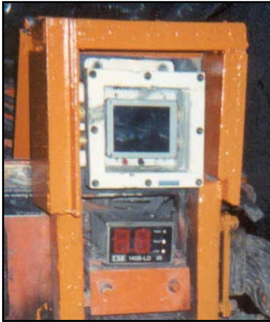
Figure 1. HS-CM system installed on a Joy 12CM12-10A and in use at Monterey Coal Company: HGU on the rear of the CM (left); Horizon Power Unit (HPU) generator within the cutter drum (upper right); Horizon Sensor Unit (HSU) on the surface of the cutter drum (lower right)
