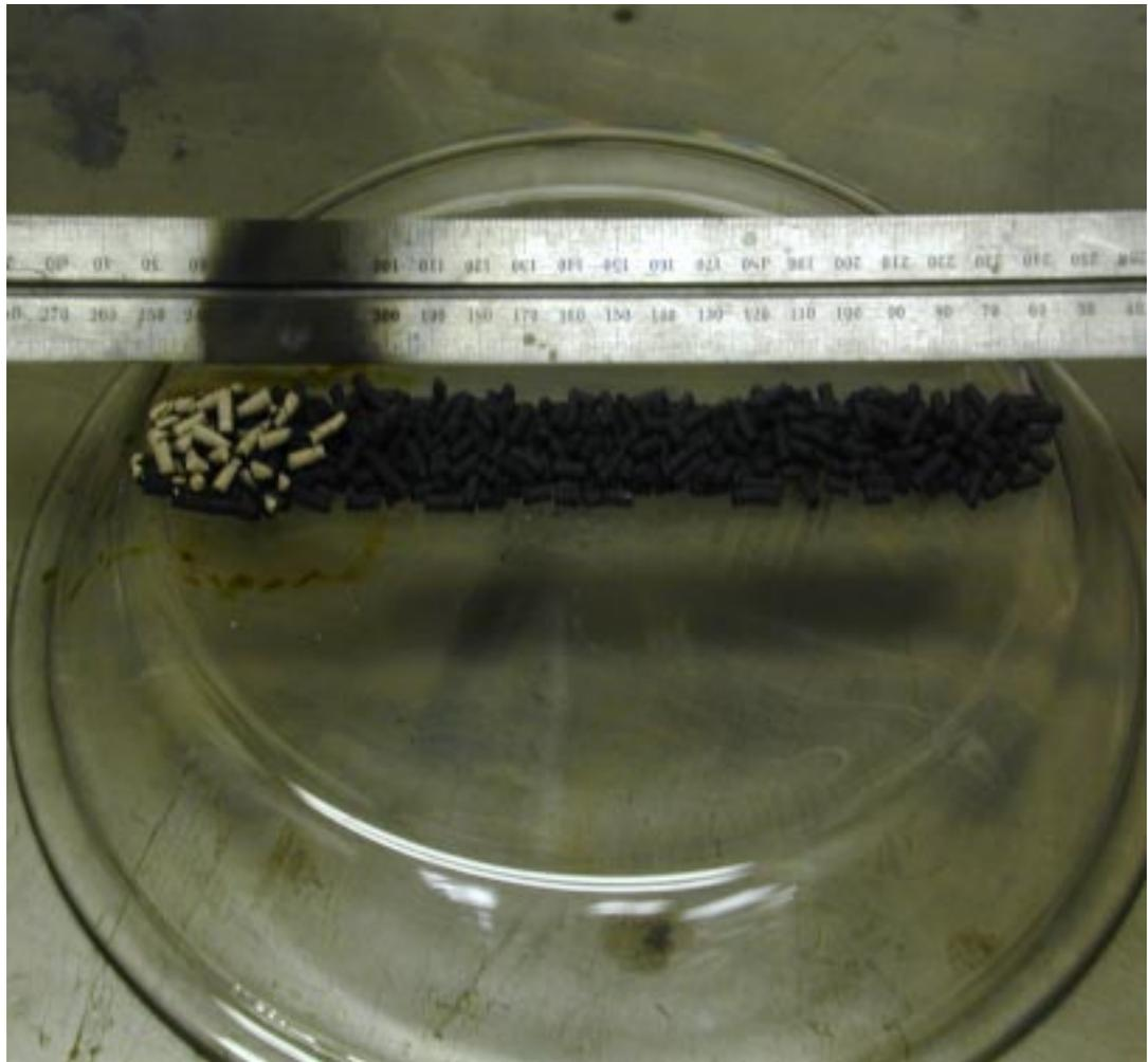
Photo #3: The pellet train after 5 min from initiation. The smolder front (a wisp of smoke can be vaguely seen) has advanced no distance from the 3.5 cm ignition zone 3 min after removal of the ignition source.
