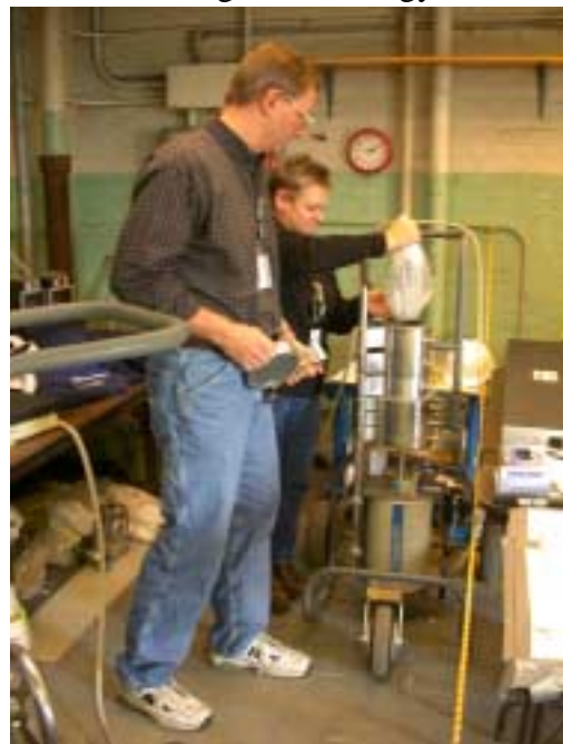
Figure 18. The ISOCS configured in the field laboratory mode for characterizing BGD soil, concrete, and debris
