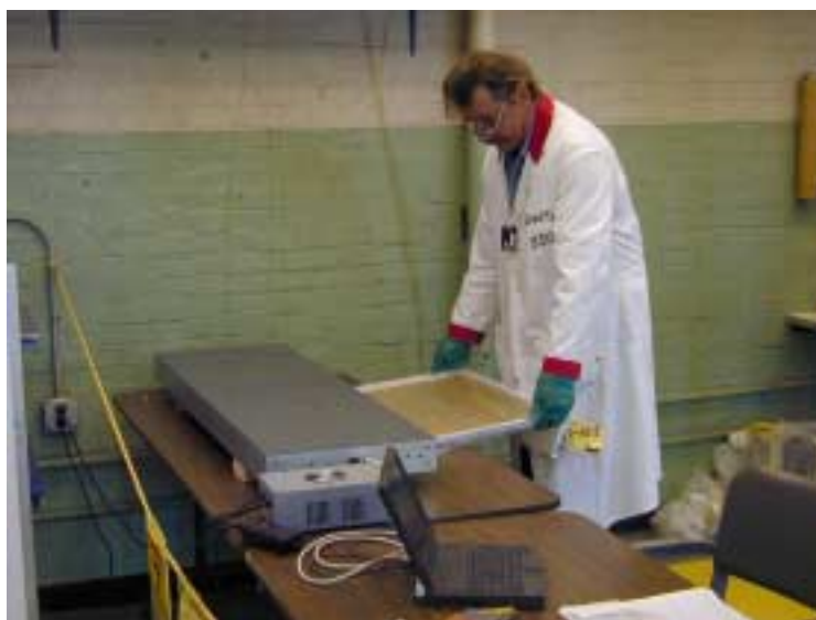
Figure 19. Loading soil samples for BetaScint characterization of Sr-90
