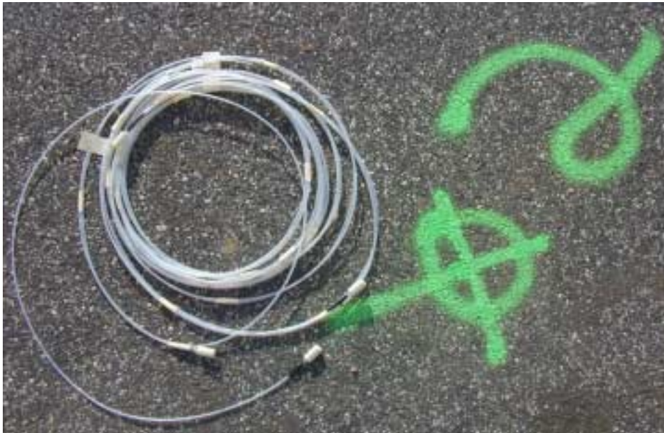
Figure 5. Bundle of sample ports showing the sintered glass filters attached to polypropylene tubing
