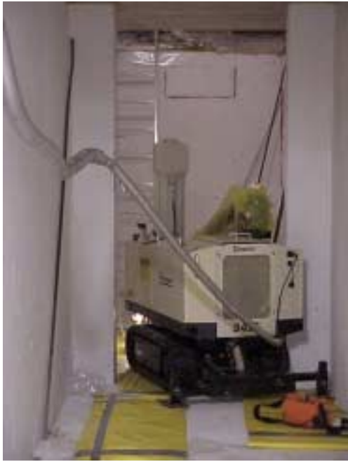
Figure 28. Geoprobe® being used in the canal deep pit
