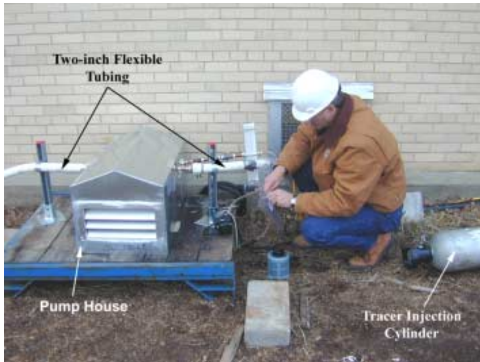
Figure 3. Pump house and flexible tubing for the North Duct circulation loop
