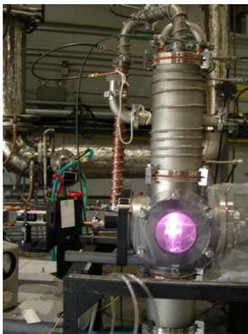
Figure 2. Photograph of the reduced-pressure air-ICP system, showing the air plasma inside the metal enclosure, part of the connection to the ICP auto-matching network (inside the wire mesh screen on the right), and the front-end of the AOTF-echelle spectrometer (on the left).
