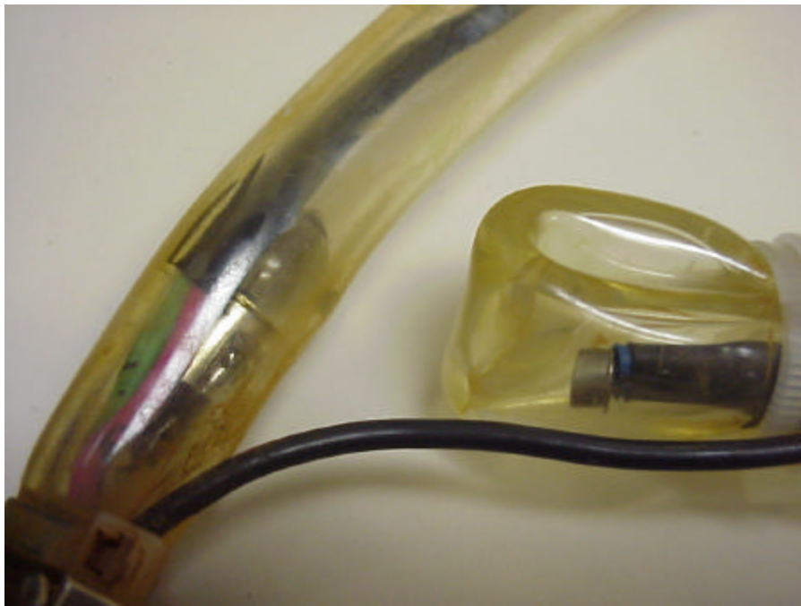
Figure 7. Photo showing details of the arrangement of the lamp and the photoresistor.
