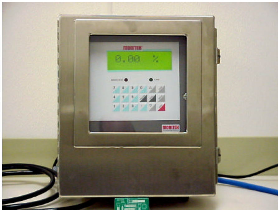
Figure 3. Photo of the Monitek Transmitter Unit housed in a NEMA enclosure.
