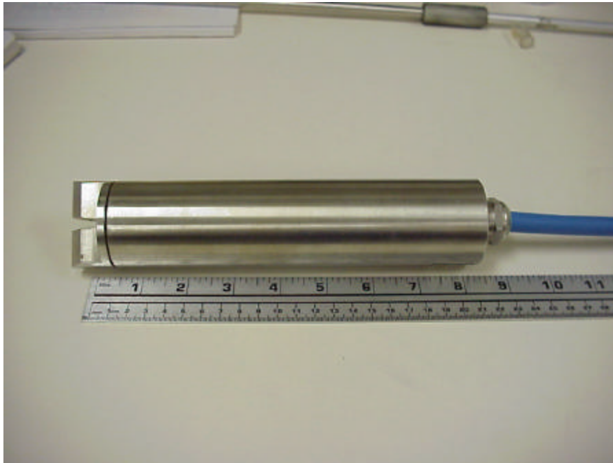
Figure 4. Photo showing the Monitek Sensor.
