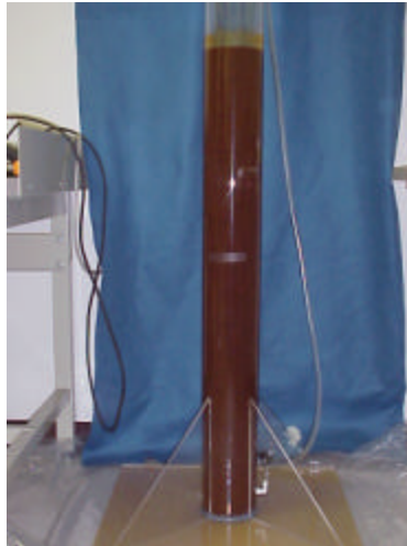
Figure 10. Photo of the test column with the sludge in a well-mixed state.
