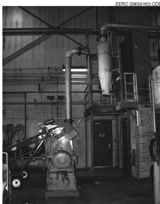
Figure 9. Photograph of the hammer mill, blower assembly, and product recovery cyclone.
