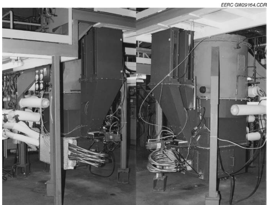
Figure 5. Photographs of the grate-fired section added to the CTF.
