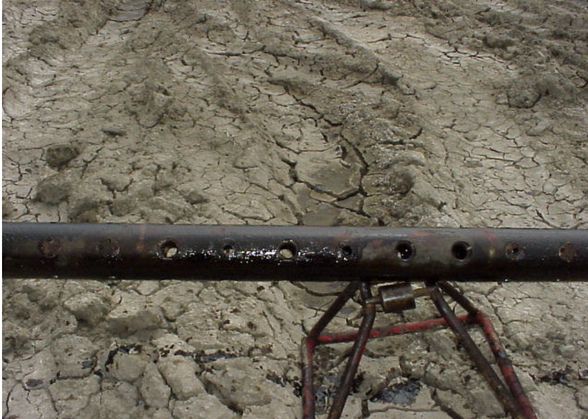
Picture 4. Well 63-TPX-10. Additional close-up of MicroFrac tool results.
