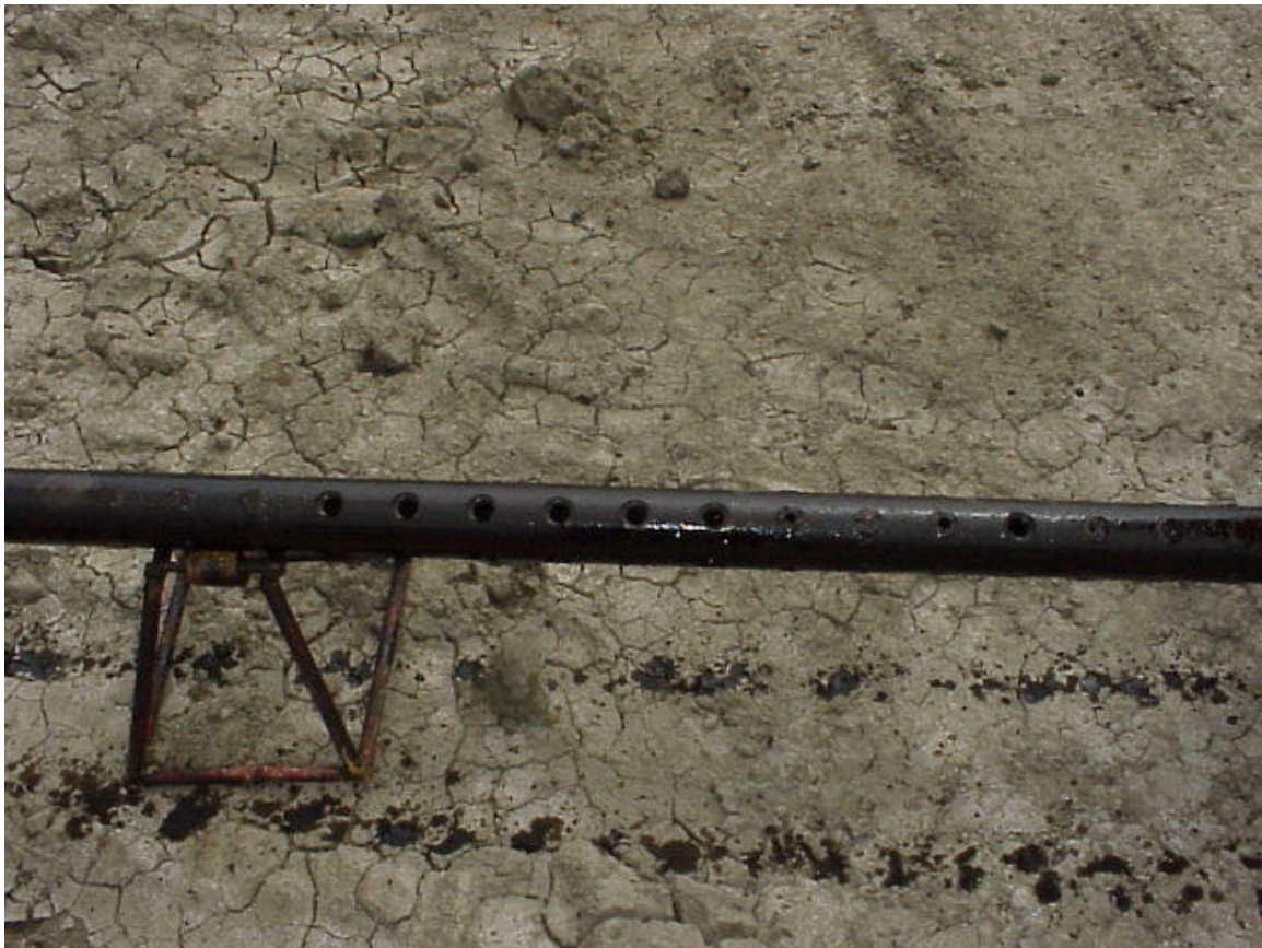
Picture 3. Well 63-TPX-10. Retrieved tool showing results of ignition. Note varying size of perforated plugs with some blown out.
