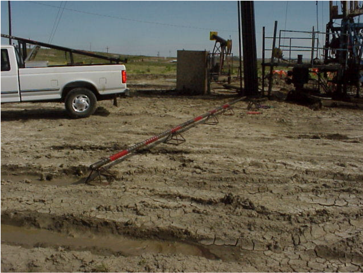
Picture 1. Well 63-TPX-10. Redesigned MicroFrac tool. Red (dark) areas on tool are propellant sections. Tool had six propellant sections.
