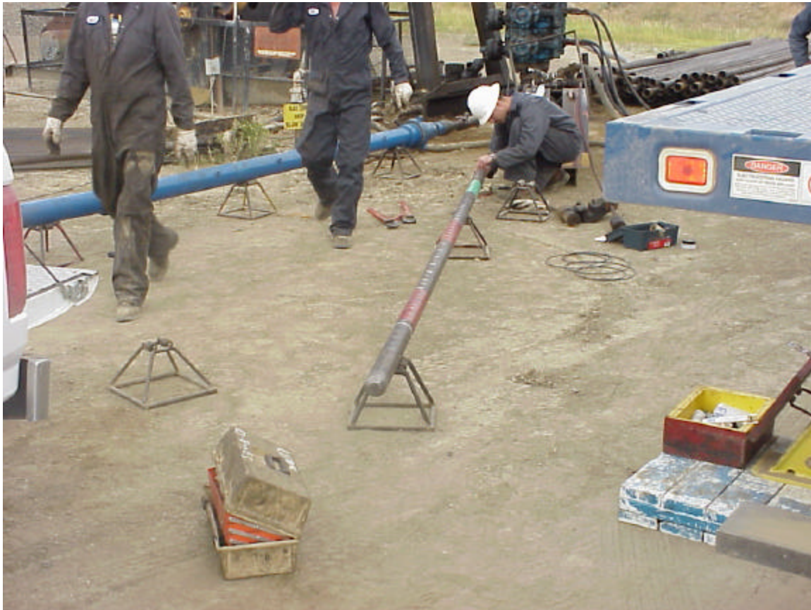
Picture 5. Well 61-A-3. First tool on second well shown being prepared for firing.
