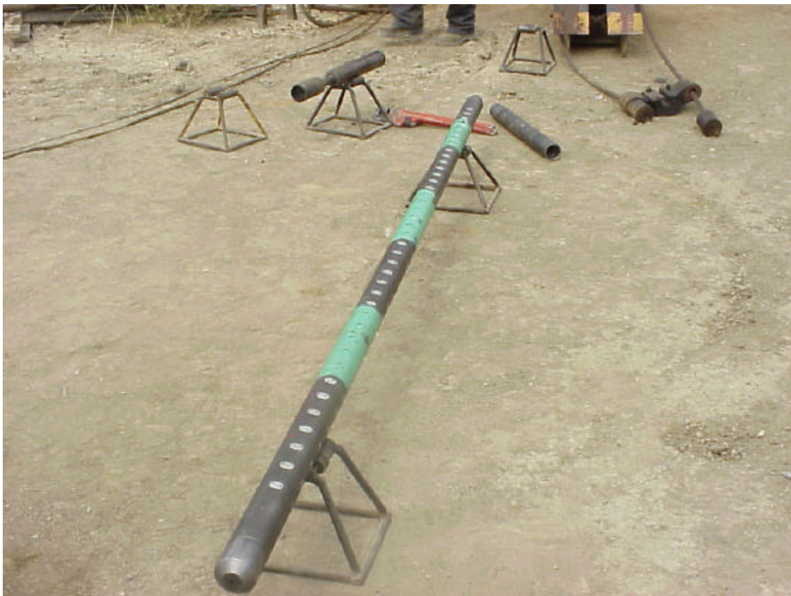
Picture 7. Well 61-A-3. Second tool being prepared for stimulation. First tool lost downhole.
