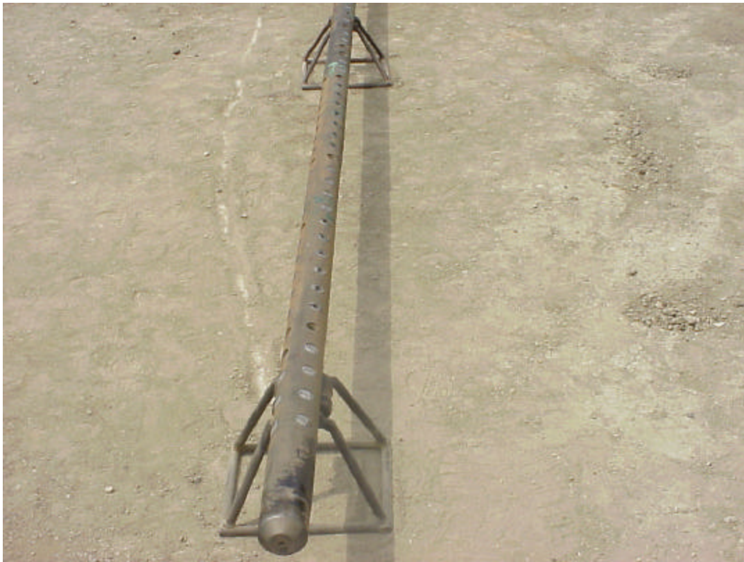
Picture 11. Well 61-A-3. Compare with Picture 7. Three rows of ports below bottom propellant section were either perforated or blown out.
