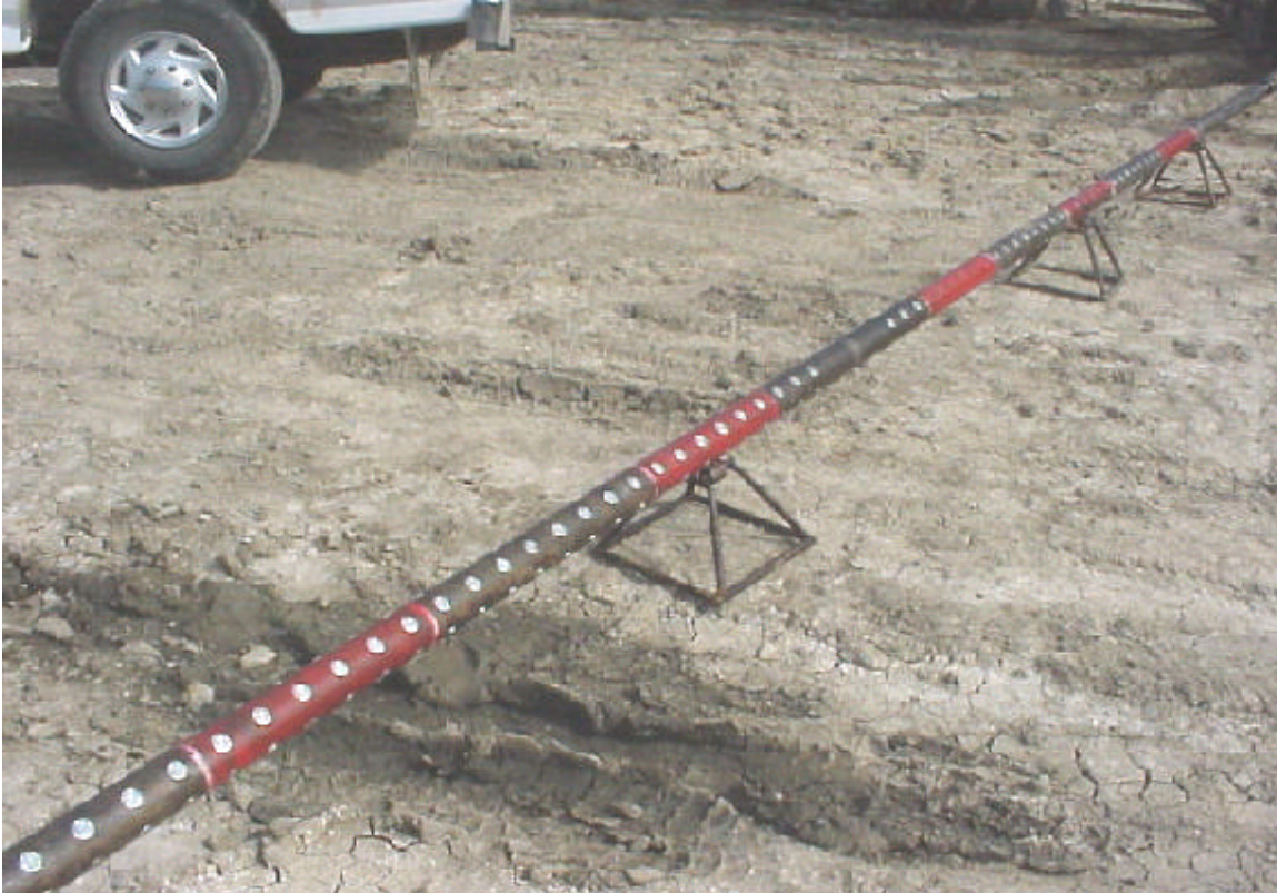
Picture 2 Well 63-TPX-10 closeup of the tool showing aluminum port plugs over propellant sections.
