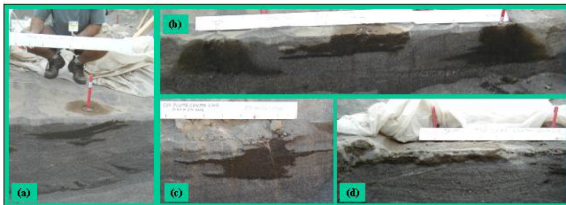
Figure 11. Typical Plumes Observed in the Field Experiment, (a) (b) and (c) show the extreme inter-bedding effects within the coarse materials, (b) the left most plume is pure water, the center 5 M NaCl, and the right 5M NaCl plus 2% methanol. The sharper, more laterally pronounced character of the saline plume was observed in almost all cases, with the methanol and water plumes generally being less sharply defined and with less vertical extent, and (d) illustrates the effect of a fine-sand layer, in which all flow is limited to the fine with complete capillary block to entry in the coarse sands.
