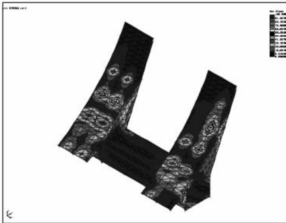
Figure 18. Von-Mises Stresses in Support Saddle.
