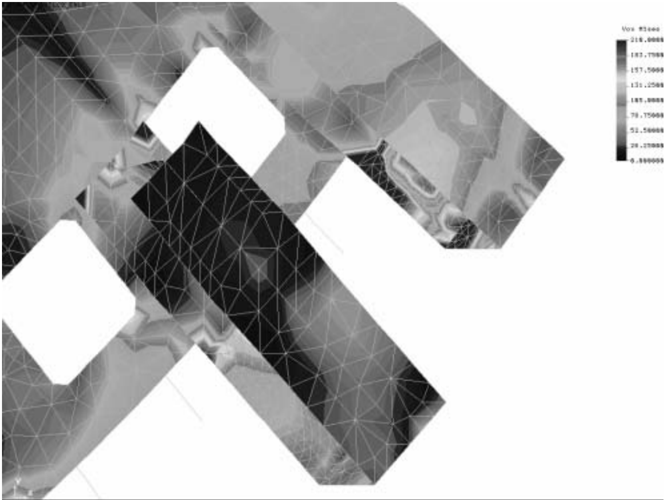
Figure 69. Von Mises Stress (Bottom) for Seismic Case F-Shell Enlarged with Scale Change (210MPa max).
