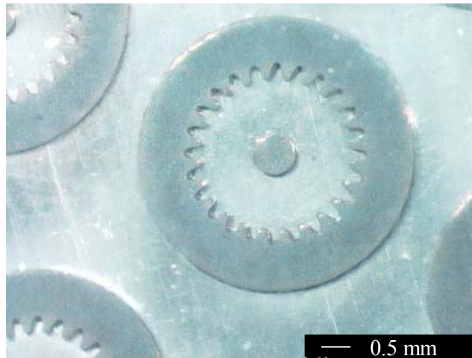
Figure 2. Optical micrographs of PMMA micro-molds with 90 μm deep cavities filled with stainless steel/epoxy: (a) top surface (b) top surface at higher magnification and (c) bottom surface taken looking through the mold.
