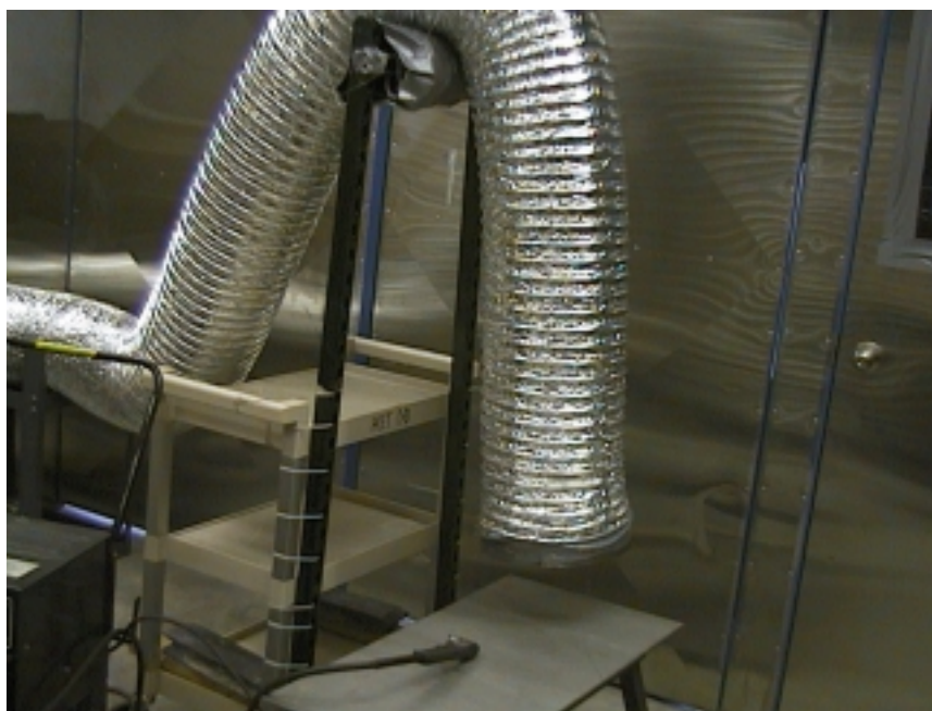
Figure 1. Arrangement for moving sampling hose over the metal to be cut.
