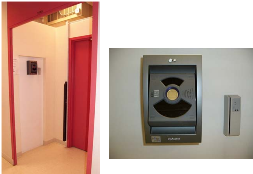
Figure 5. Alcove Installation of the Remote Unit (left) and Closeup (right)
