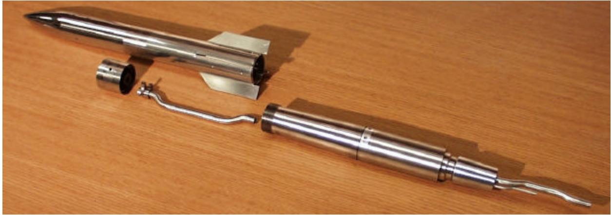
Figure 21 A view of the assembled model along with the spin rig, a nozzle section, and pressure tubing to supply the secondary gas supply to the jets.
