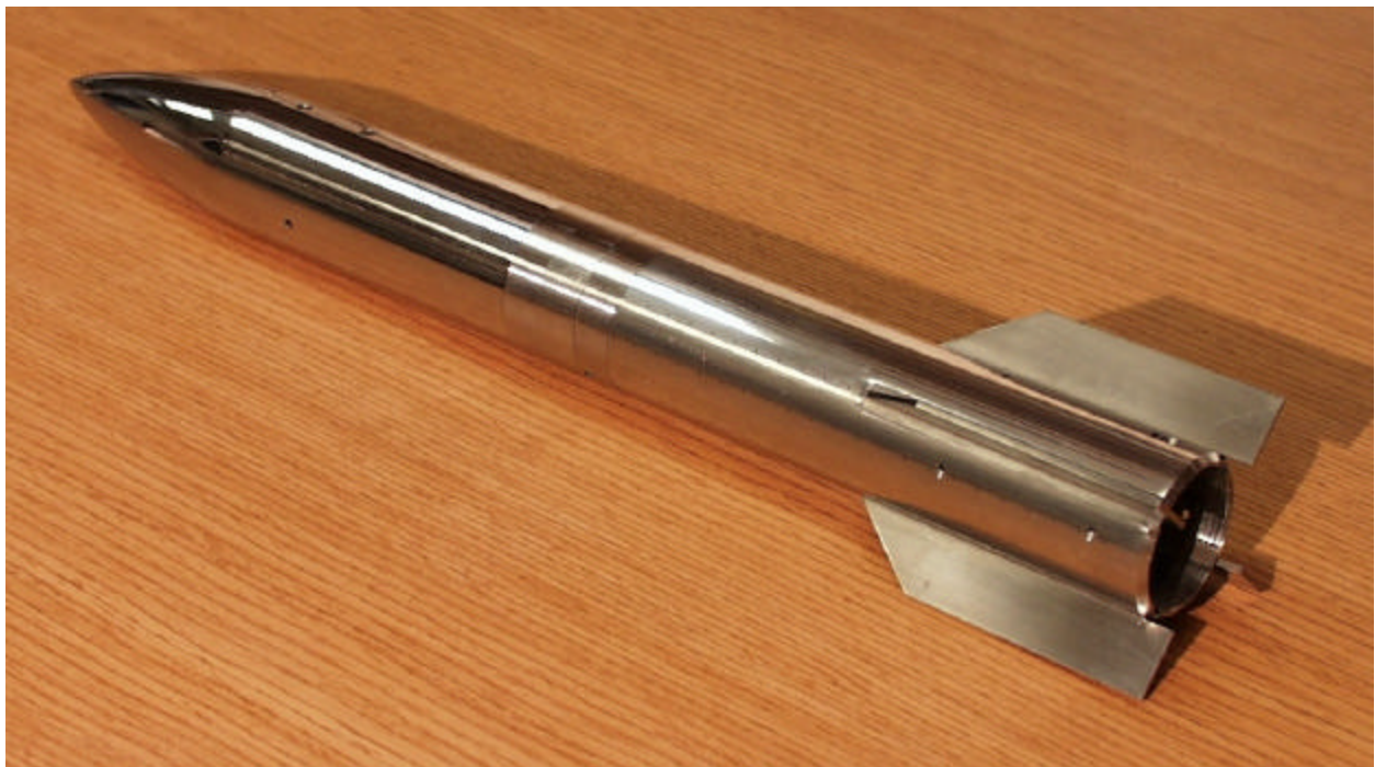
Figure 20 A fully assembled view of the innovative wind tunnel model, using the same parts shown in the photograph of Figure 19 (except for the fin retaining ring).
