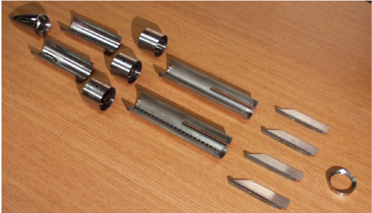
Figure 19 Disassembled view of the innovative wind tunnel model.
