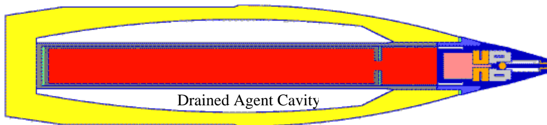
Figure 3. CTH model representation of the drained M121A1 155 mm chemical round with T244 fuze. (Munition case material is shown in yellow, burster and booster charges are red, and fuze charge is pink.) The overall length of the projectile, with the fuze present, is 69.8 cm (27.5 in).
