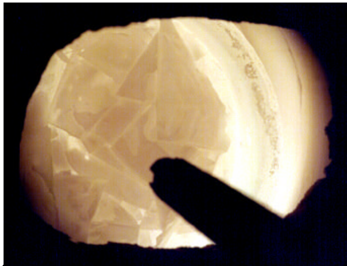
Fig. 4. Production casting furnace showing emissivity variation on the melt and a hot crucible.
