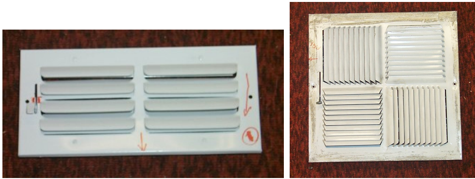
Figure 3. Examples of registers used in flow hood test apparatus
