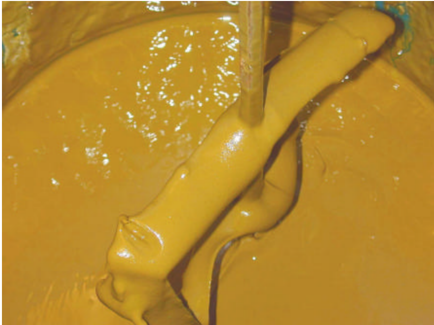
Figure 4 MER04 Sludge Surrogate Prior to SPSS Treatment.
