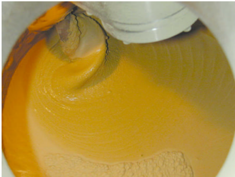
Figure 8 MER04 Sludge With Partial SPC, After 5 min Mixing.
