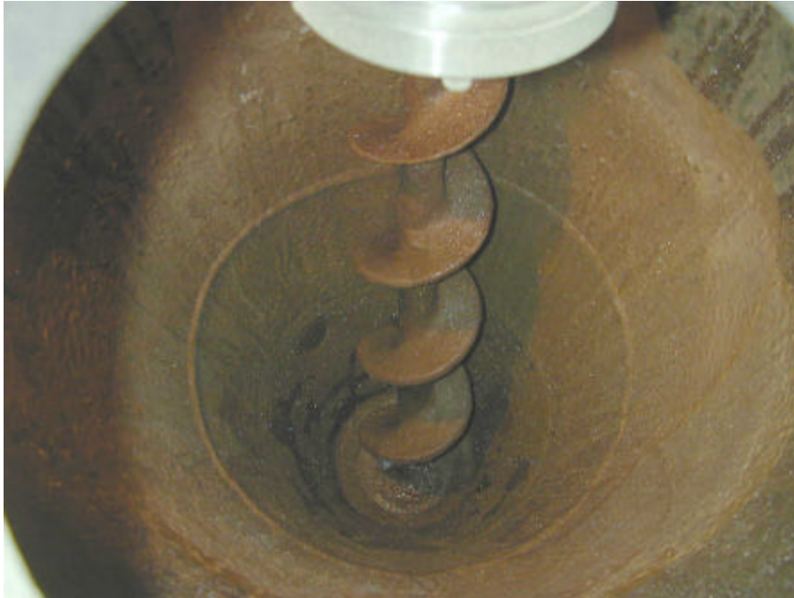
Figure 5 Inside View of Vertical Cone Mixer.
