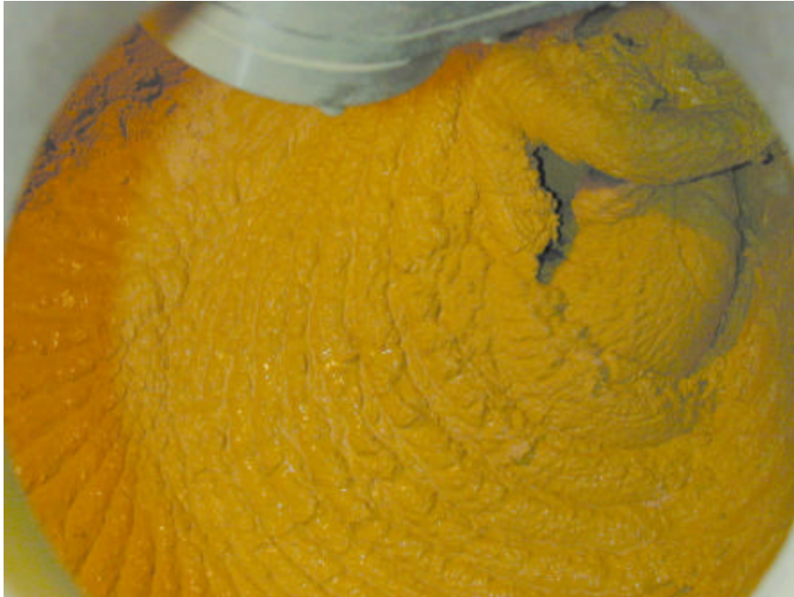
Figure 7 MER04 Sludge With Partial Quantity of Powdered SPC.
