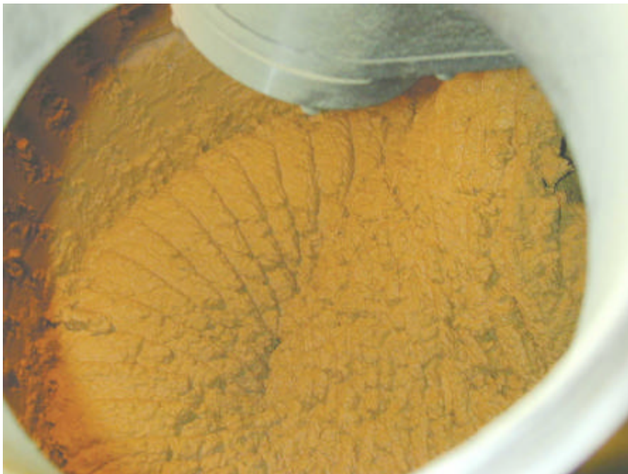
Figure 10 MER04 Sludge With Balance of SPC, After 5 min Mixing.
