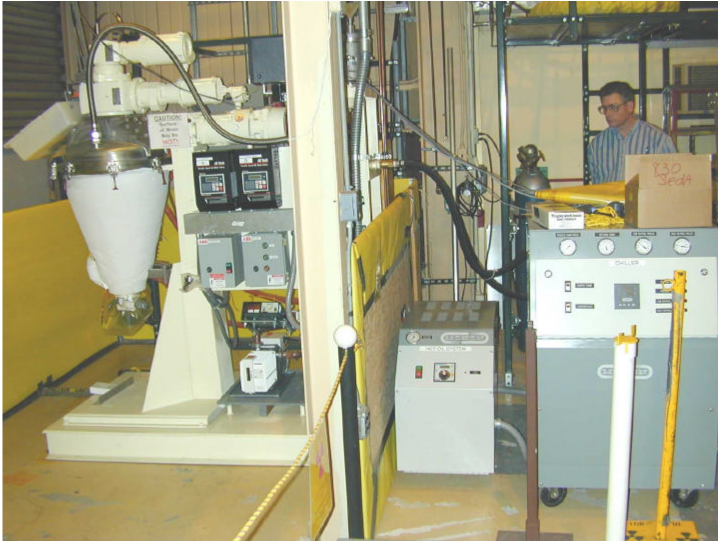
Figure 1 SPSS Vertical Cone Mixer and Process Controls.
