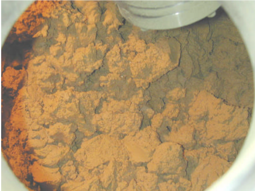
Figure 9 MER04 Sludge, After Adding Balance of Powdered SPC.
