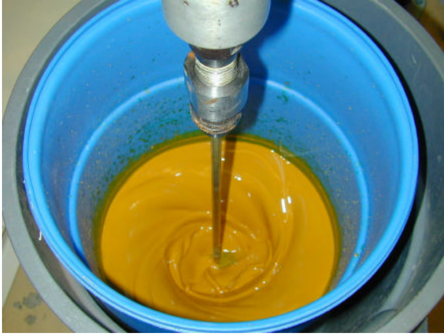
Figure 3 MER04 Sludge Surrogate Preparation.
