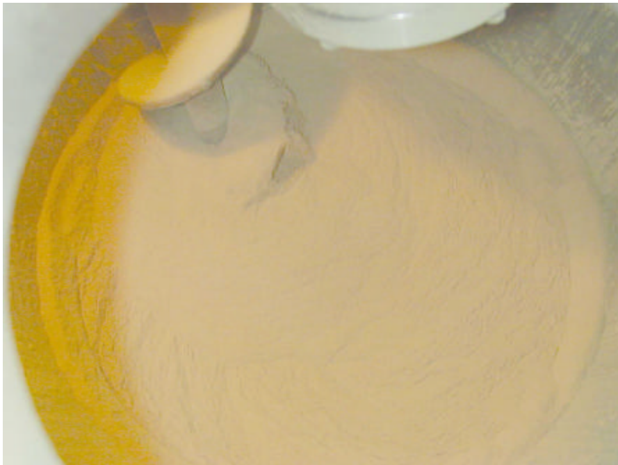
Figure 6 Powdered SPC Added to Vertical Cone Mixer.
