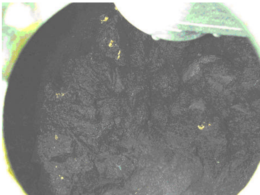
Figure 12 MER04 Sludge/SPC Mixture, After Complete Addition of \text{Na}_2\text{S} .
