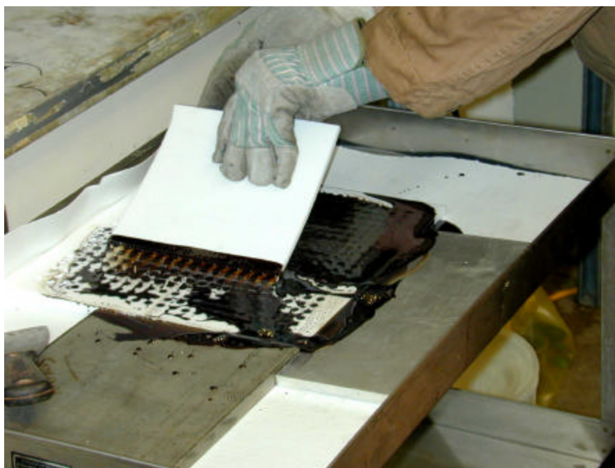
Figure 15 Preparation of TCLP Pellets from SPSS Treated MER04 Sludge.
