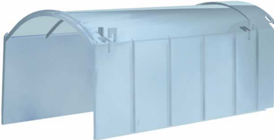
Figure 4. Drip Shield Isometric View
