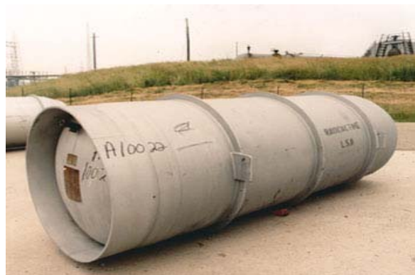
FIGURE 1.1 Typical 12-metric-ton Depleted \text{UF}_6 Storage Cylinder
