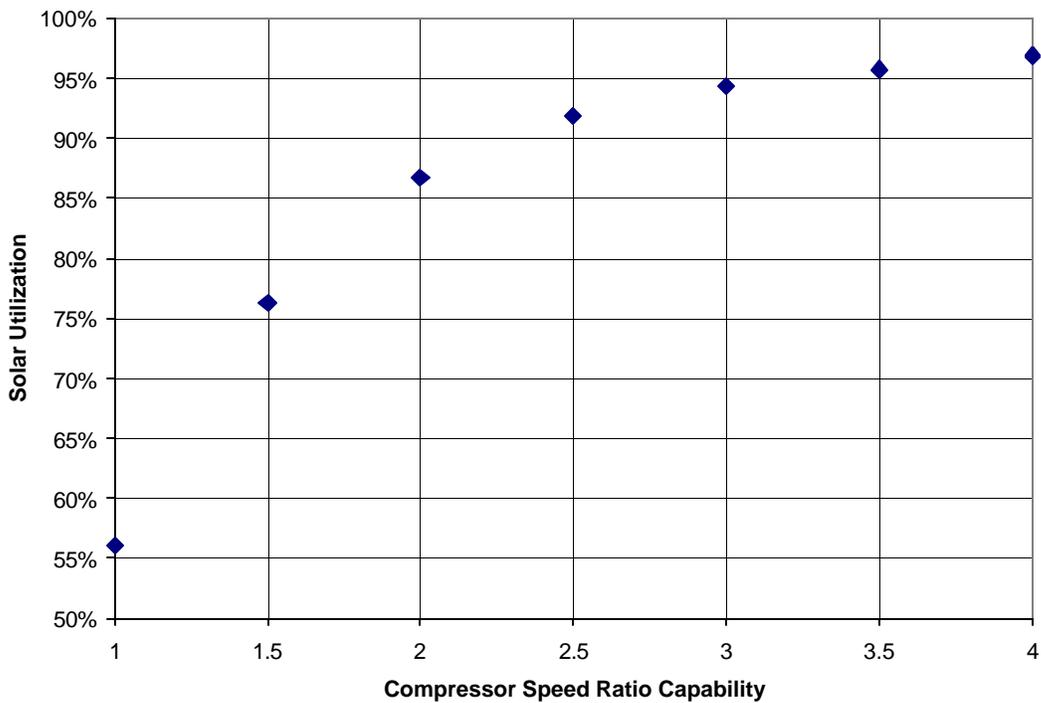
**Figure 3. Solar Utilization with Different Speed Ranges**
