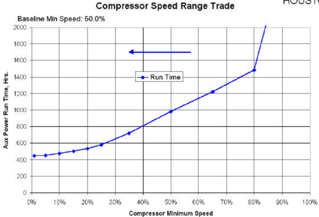
**Figure 25. Compressor Speed Range vs. Run Time (Houston)**
