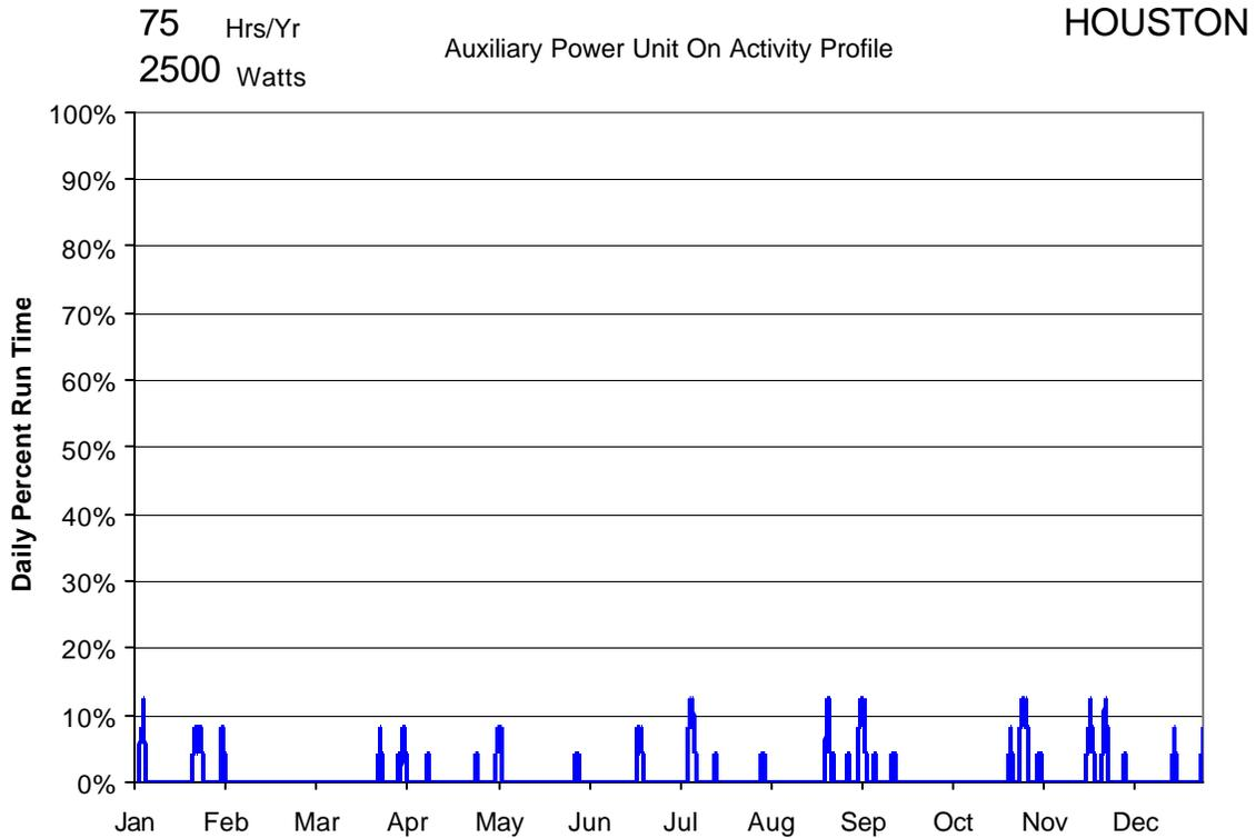
**Figure 22. Auxiliary Power Use Profile**
