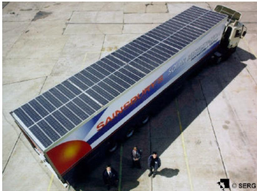
**Figure 1. Solar PV Refrigerated Trailer**
