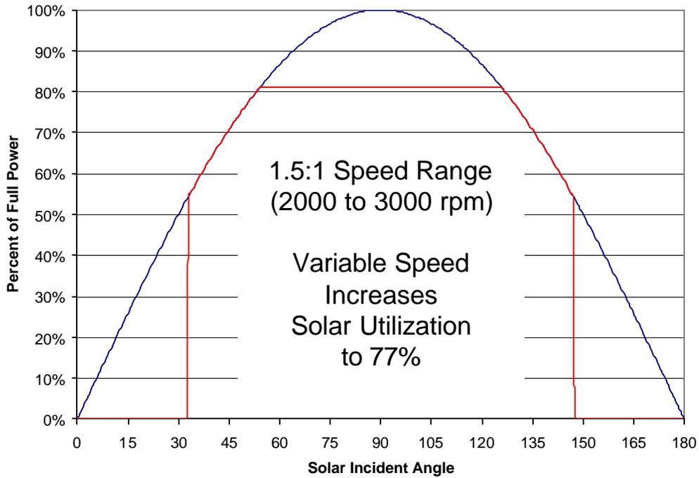
**Figure 2. Solar Utilization with 1.5:1 Speed Compressor**
