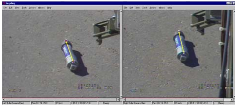
Figure 5. Using Visual Targeting and Active Sketch the operator indicates position, orientation and location for the robot to grasp a pipe.
