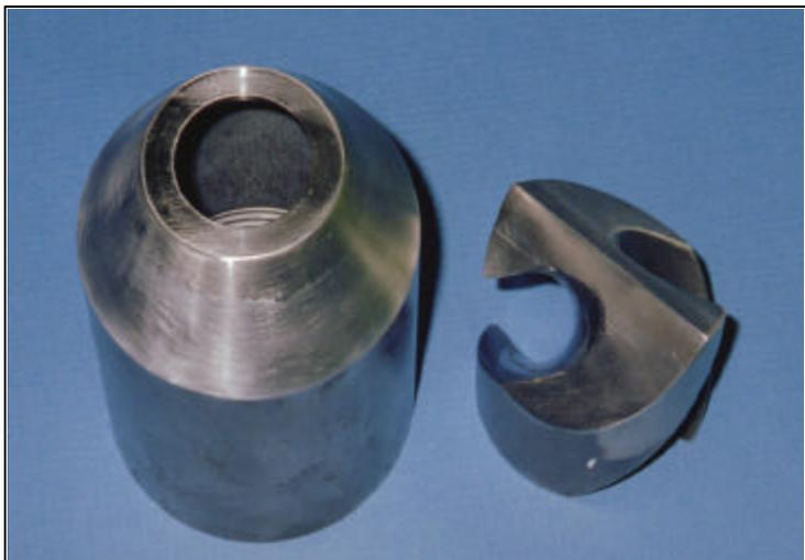
Fig. 2 Splash plate and swirl type liquor nozzles after application of iron aluminide. steel plate and then overlaid with a pad of iron aluminide weld metal. The plates were installed in a mill in the south central U.S. and their performance monitored by periodic visual examinations by mill personnel.
