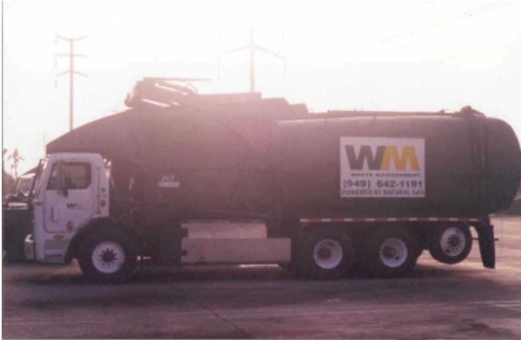
**Photo 5-5. Left-hand View of WMI Trash Truck Following the Retrofit with a 280 HP John Deere 8.1L CNG Engine**
