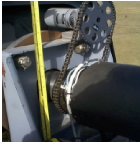
Figure 38. Azimuth angle encoder photograph and orientation
