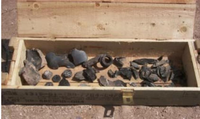
Figure 27. Debris from Two Low Order Detonations
