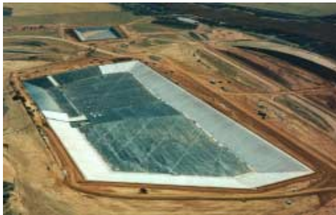
Figure 3. Aerial view of the double composite-liner system at the base of the repository.
