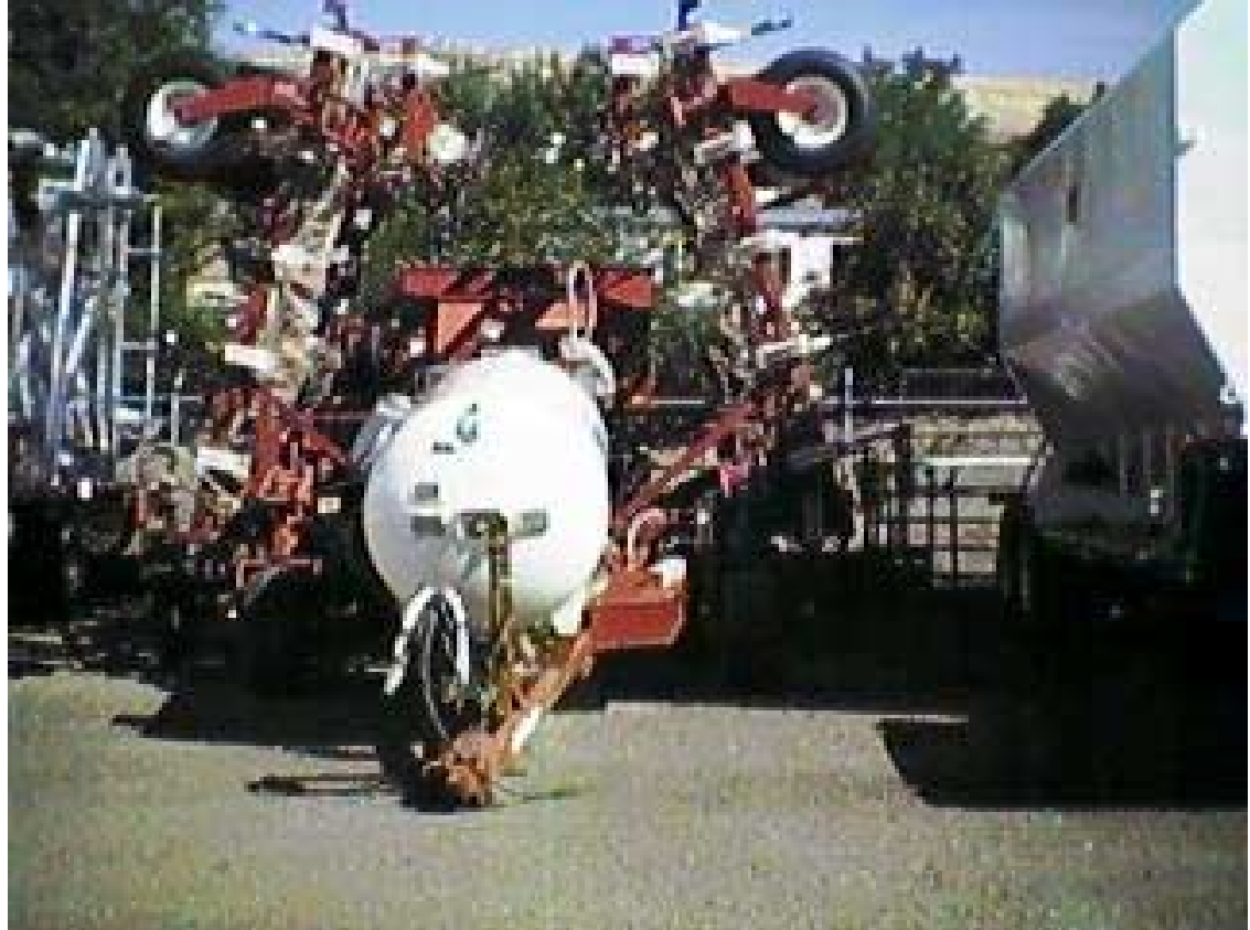
Figure 2 Straw Boss fertilizer applicator
