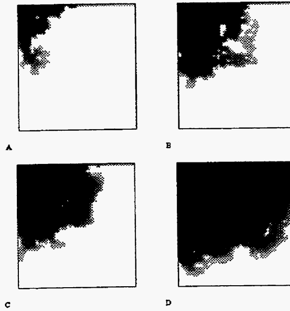
Figure 11 Concentration patterns for run 4 at the four different occupation fractions. Darker colors indicate smaller concentrations. Pe=331 , Q=0.25 \cdot 10^{-6} \text{ m}^3/\text{s} .
