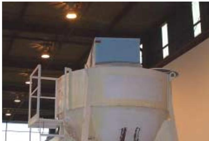
**Figure 12: Dust Containment Box on Dry Goods Silo**
