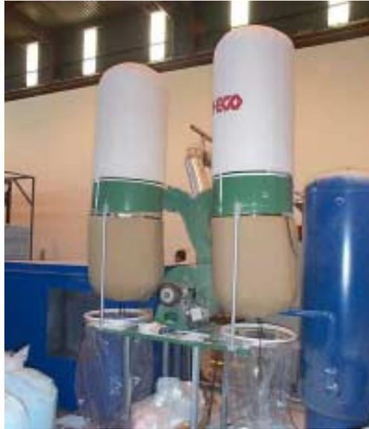
**Figure 11: Modified XPS Dust Collection System**
