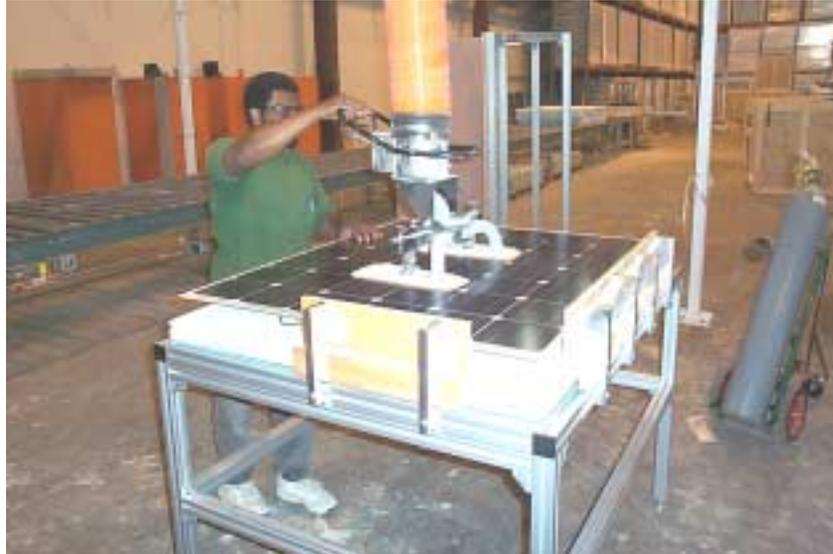
**Figure 2: PV Laminate Placed on Backerboard**
