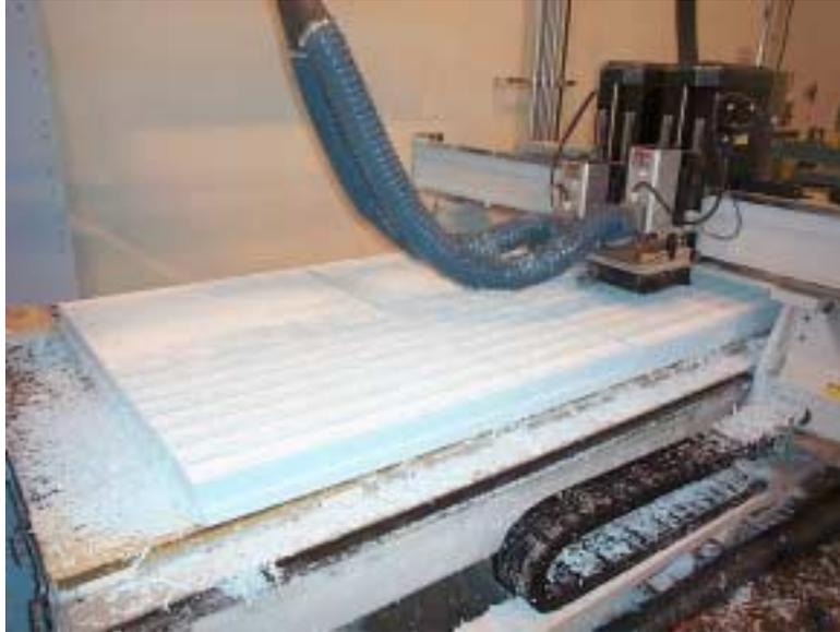
**Figure 1: Spacer Cutting with CNC Router**
