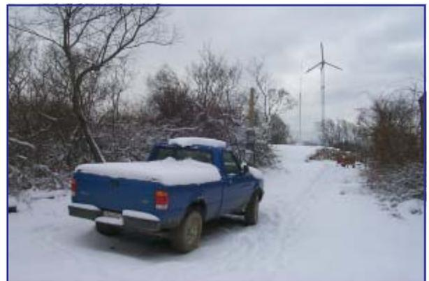
*Figure 5. This Ford Ranger electric vehicle is charged with excess wind energy from a Bergey Excel 10-kW wind turbine.*
