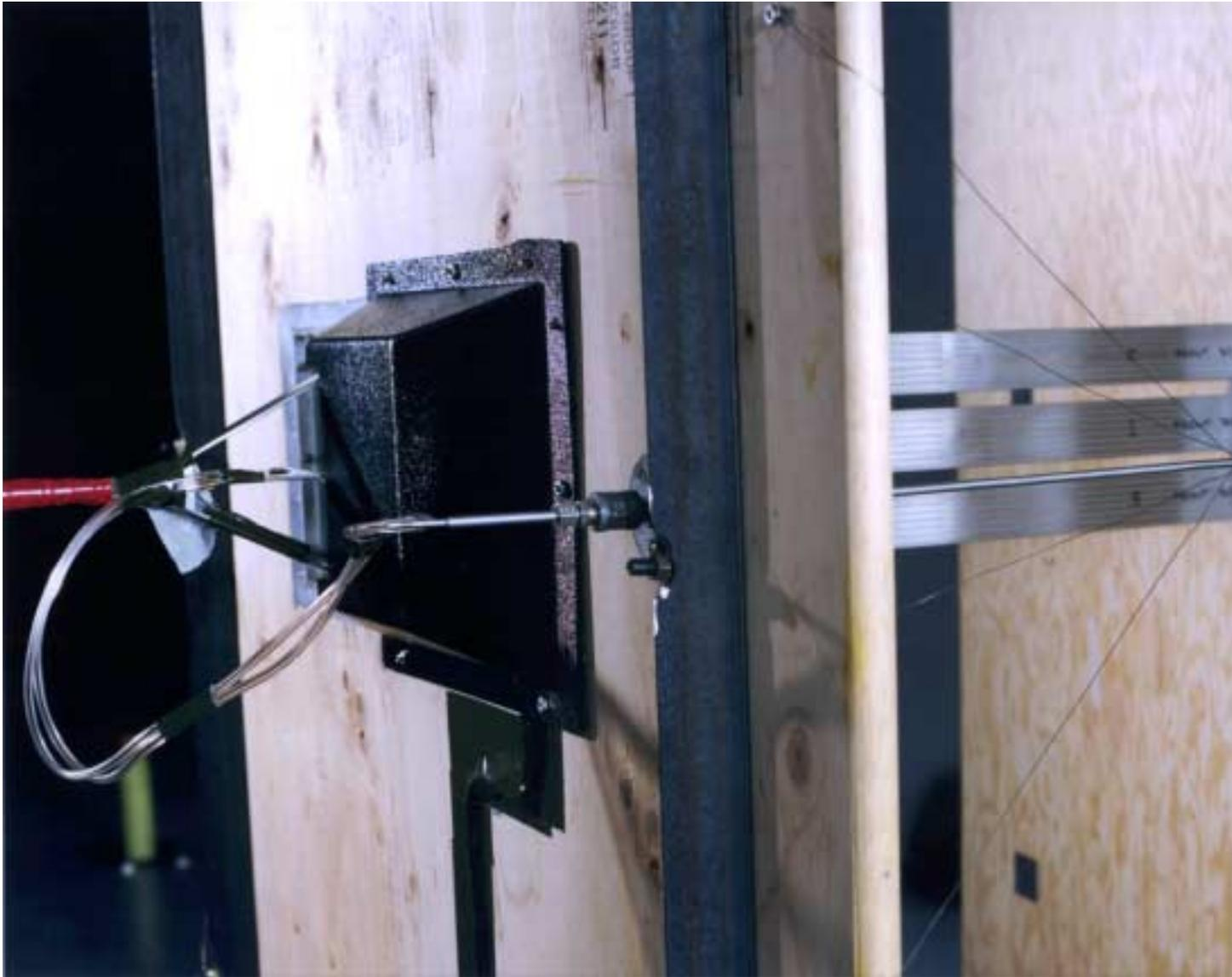
Figure 7. Photograph of windshield covering pressure transducers and connections.
