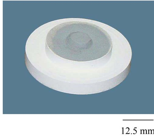
Figure 6 Blank of cermet inside mold before firing at 1650°C.
