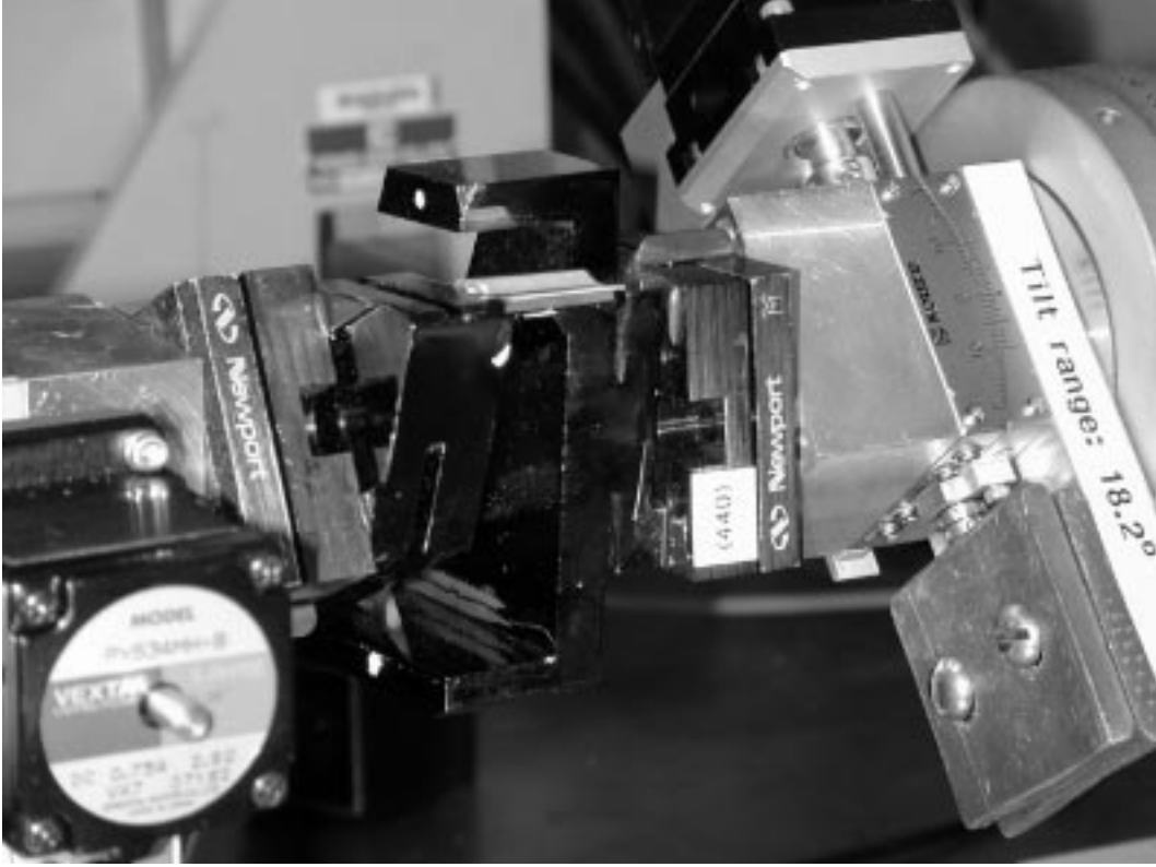
Figure 6: Picture of the high-resolution monochromator. The (4 4 0) channel cut is mounted on the right rotation stage. The incident x-rays are reflecting off the lower side (not visible) of the top silicon piece. The monochromatic beam leaves the device from the low lying surface of the same channel cut.
