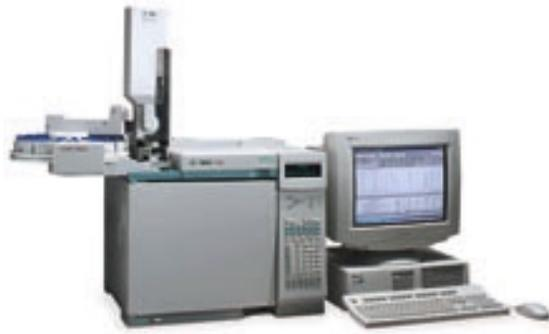
**Figure 1. Agilent 6890 Gas Chromatograph.**
