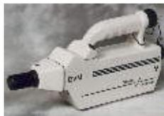
**Figure 2. Femtoscan portable GC/IMS instrument.**
