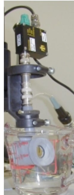
Figure 8. Sandia TSM resonator sensor shown in a liquid bath during the viscosity testing.
