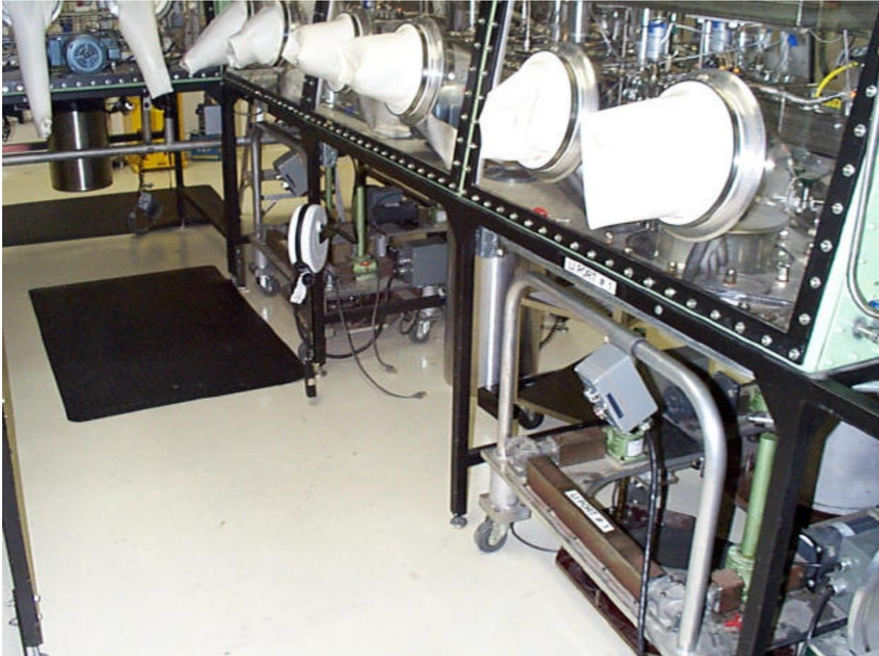
This mounting configuration results in a relatively flexible system. The lack of bracing in the glovebox legs introduces some flexibility into the system. In addition, all of the support legs are not anchored. Finally, it was noted that there are a large number of penetrations entering the gloveboxes. These penetrations are necessary for processes. The umbilicals entering the penetrations are generally attached to adjacent gloveboxes in the same line, or to remote locations.
