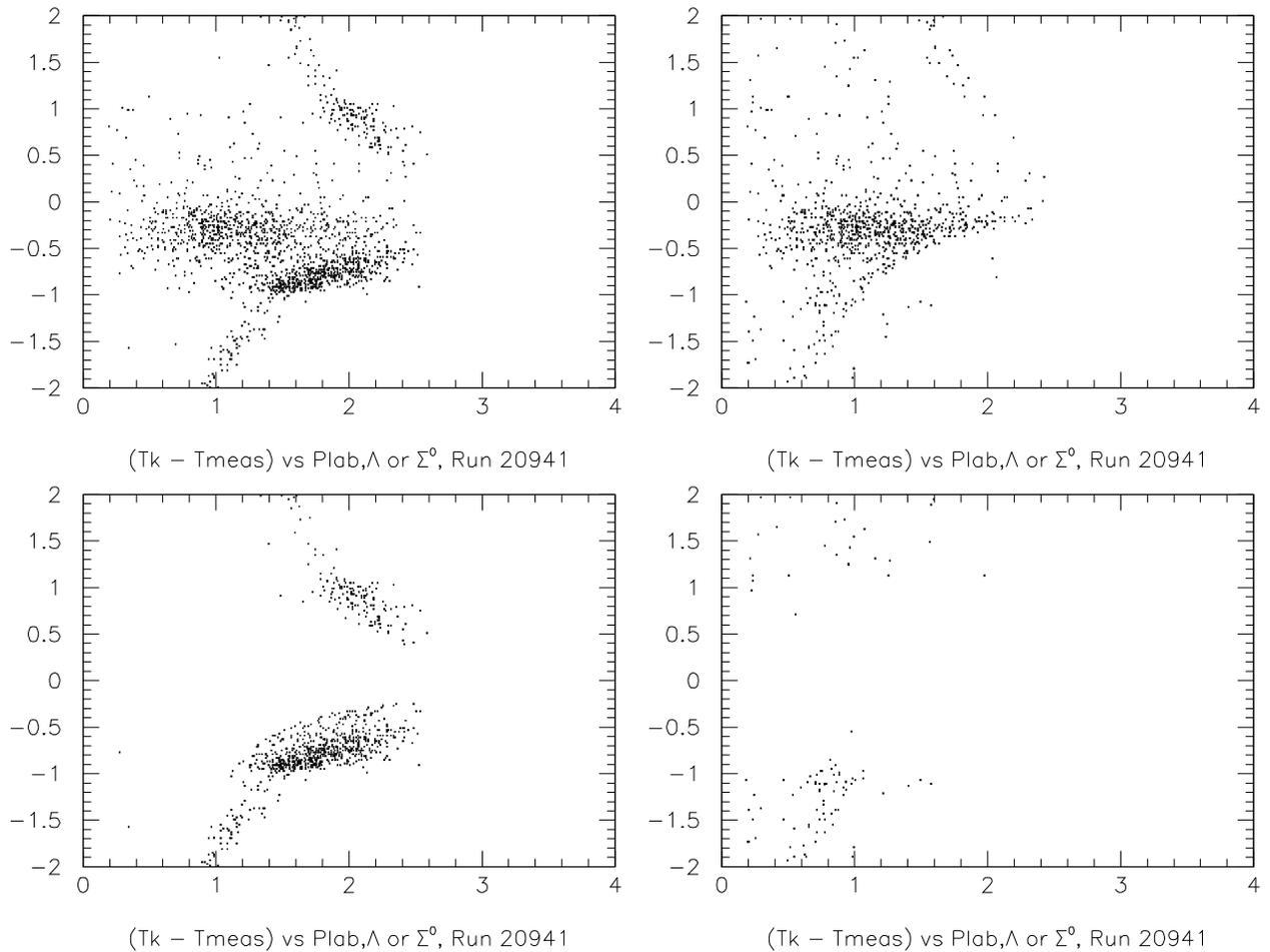
Figure 2: Time difference between measured particle ToF and hypothesized kaons of a given momentum vs lab momentum. Only particles where the missing mass is consistent with a  $\Lambda$  or  $\Sigma^0$  were plotted. The upper left and right panels show the Ktof and K filters respectively. The lower left panels show events that passed the Ktof filter and were rejected by the K filter. The lower right panel shows events that passed the K filter and were rejected by the Ktof filter.
