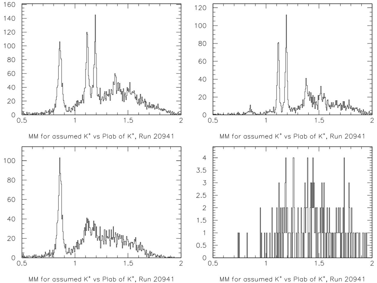
Figure 4: Missing Mass assuming Kaon for “good” kaons . The upper left and right panels show the Ktof and K filters respectively. The lower left panels show events that passed the Ktof filter and were rejected by the K filter. The lower right panel shows events that passed the K filter and were rejected by the Ktof filter. Note the peaks around 1.1 GeV in the (Ktof and not K) panel on the lower left which shows that the new filter preserves some kaon events rejected by the old filter.
