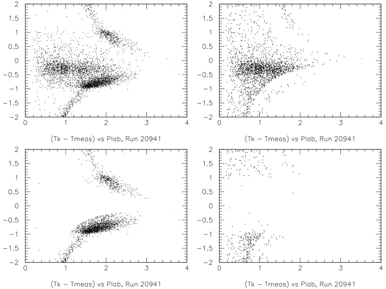
Figure 1: Time difference between measured particle ToF and hypothesized kaons of a given momentum vs lab momentum. The upper left and right panels show the Ktof and K filters respectively. The lower left panels show events that passed the Ktof filter and were rejected by the K filter. The lower right panel shows events that passed the K filter and were rejected by the Ktof filter.
