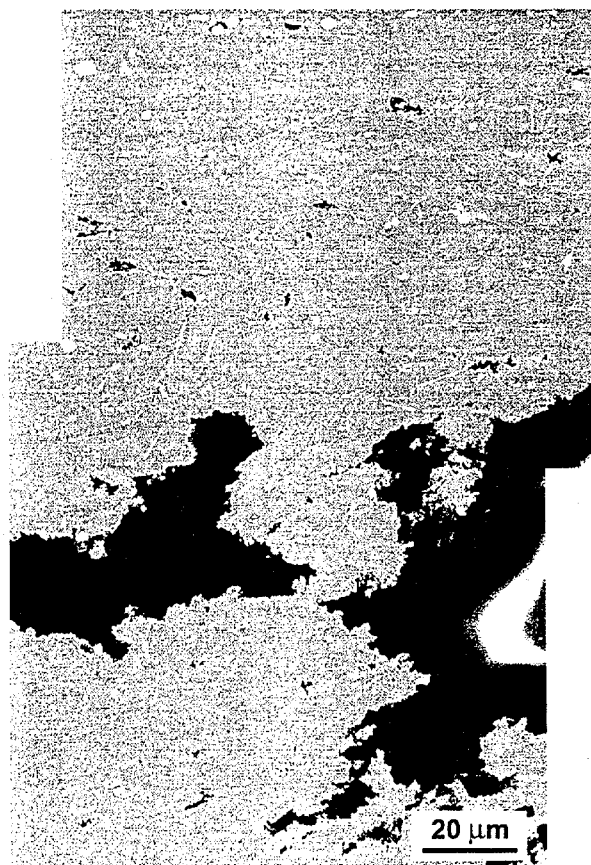
Fig. 6. Scanning electron micrographs showing creep cavitation in a Haynes 25 specimen aged at 850°C for 2015 h and tensile tested in vacuum at 750°C at a strain rate of 3.3 \times 10^{-5} \text{ s}^{-1} : (a) low magnification of longitudinal section of tensile-tested specimen, (b) higher magnification of region enclosed in box.
