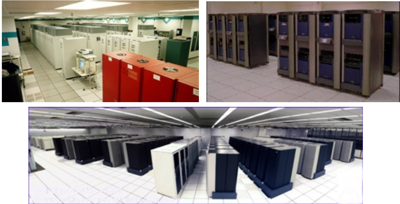
Figure 11. ASCI has brought about development and installation of three of the world's fastest computer platforms. Intel's ASCI Red machine (upper left), located at Sandia Albuquerque, was the world's first teraOPS computer and was recently upgraded to more than three teraOPS. ASCI Blue Mountain (upper right) was installed at Los Alamos by SGI and has achieved a peak speed of over three teraOPS. ASCI Blue Pacific (bottom) was installed by IBM at Lawrence Livermore and has also broken the three-teraOPS barrier.
