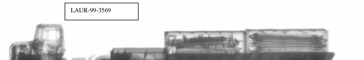
Figure 6 VACIS™ Image of Crates Containing Piping
