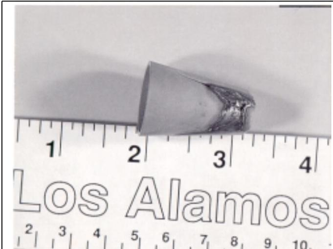
ZSBN ceramic alloy exposed to molten Be for 30 minutes at 1350° C.
