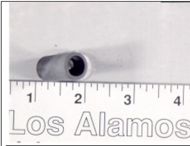
$ZrO_2$  crucible exposed to molten Be for 15 minutes at  $1400^\circ C$ . The beryllium stuck to the inside of the crucible. The Be separated from the crucible during cross sectioning indicating less reaction than in the case of yttria.
