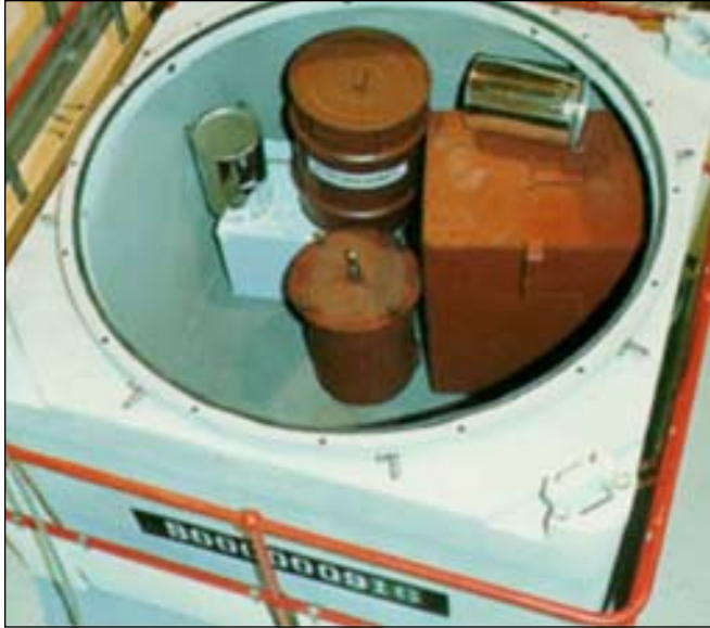
Figure D-8.3. Waste Disposal Container as it is being Filled
