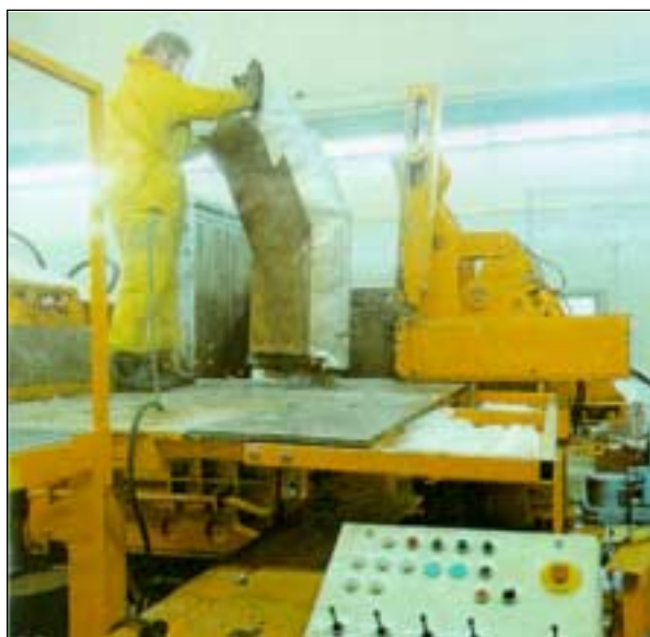
Figure F-1.1. Scrapping Press in the Caisson; the Pressing Force is 337,000 lbs/ft
