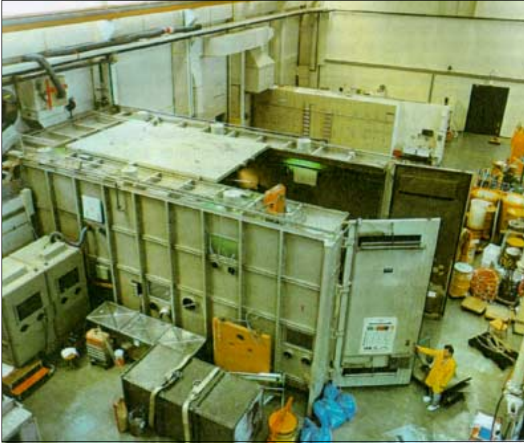
Figure F-1.3. Large Caisson in which Dismantled Plant Components are Decontaminated
