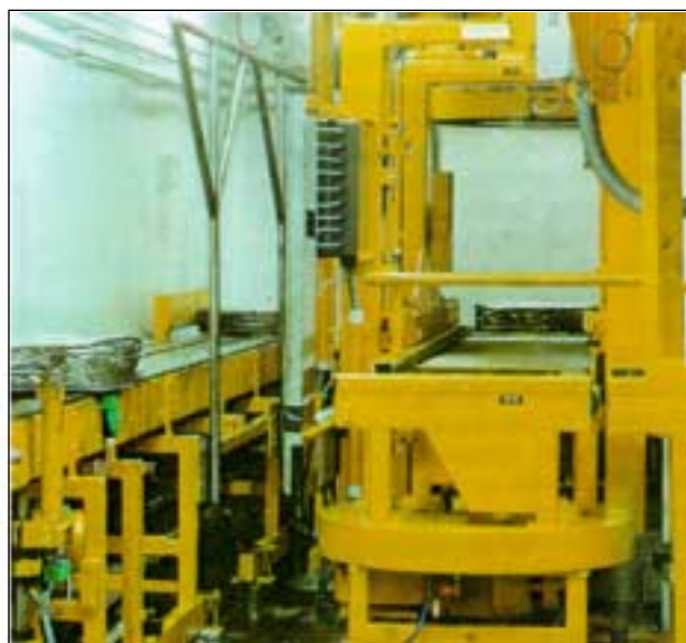
Figure F-1.2. High-Pressure Press with Transport System. The Pressing Force is 3,370,000 lbs/ft
