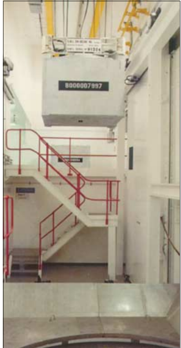
Figure D-8.4. Full Waste Disposal Container being Transferred to where it will be Stacked on a Stool
