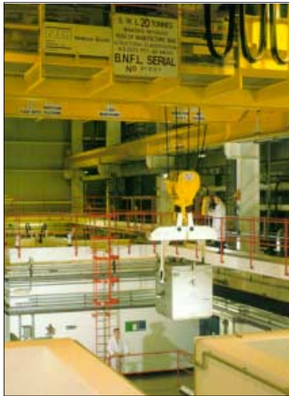
Figure D-8.2. 20-Tonne Crane Moving a Loaded Flask
