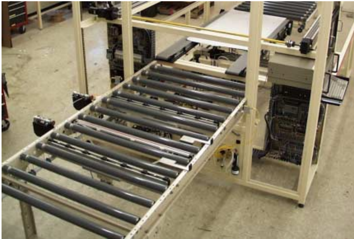
Figure 31 Input conveyor and aligner.
