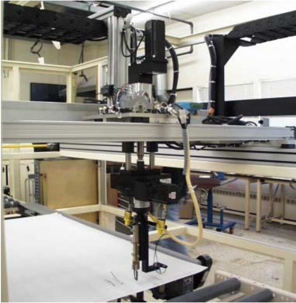
Figure 33 Edge trimmer robot and end-effector.
